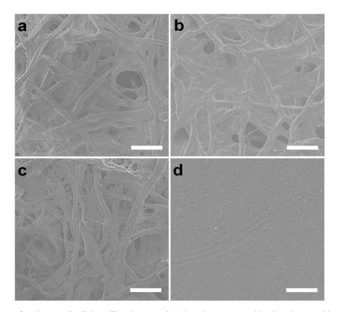
**Figure S1.** Surface image of cellulose fiber in paper showing changes caused by the photocurable resin during 3D digital light printing (DLP) and ethanol washing. (a) The bare filter paper. (b) The filter paper soaked with resin. (c) 10 times of ethanol washing after the filter paper was soaked with resin (d) The fully cured paper. (Scale bar: 50 µm. magnification: 100X). Images were obtained with Scanning electron microscopy (JSM-6700F, JEOL, Tokyo, Japan).
