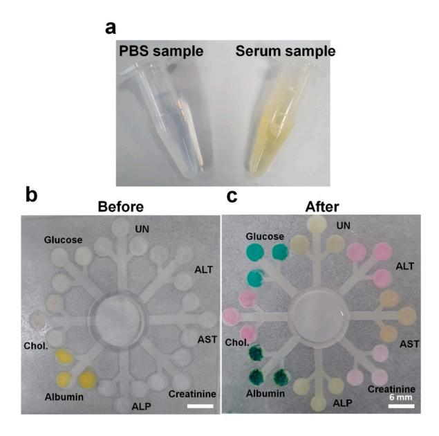
**Figure S2.** Multiple detection on the 3D- $\mu$ PADs using a serum sample. (a) Color difference between the PBS sample and spiked serum sample in tubes. (b) Each enzyme was fixed on each detection zone before testing. (c). Detection of multiple biomarkers by dropping the sample (300  $\mu$ L) including 8 mmol/L for glucose, 8 mmol/L for Chol., 4 g/dL for albumin, 400 U/L for ALP, 150  $\mu$ mol/L for creatinine, 400 U/L for AST, 400 U/L for ALT, 4 mmol/L for UN in spike serum sample.
