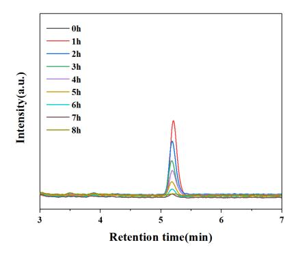
Figure S2. High performance liquid chromatography of phenol peak during degradation by CTAB-TCPP.
