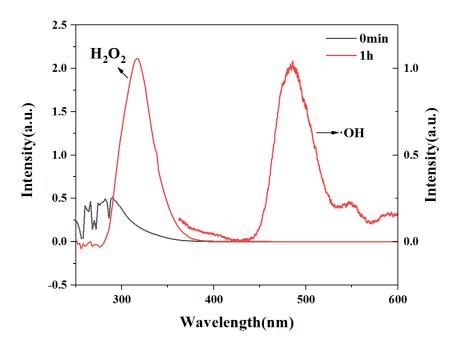
Figure S6. the UV-vis adsorption spectra and PL spectra of titanium (IV) oxysulfate and coumarin for detection of H<sub>2</sub>O<sub>2</sub> and •OH.
