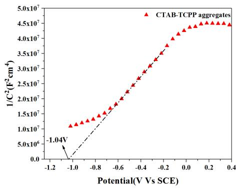
Figure S4. The Mott-Schottky plots of CTAB-TCPP aggregates. The frequnze of 1000 Hz was used to detect the flat band position.
