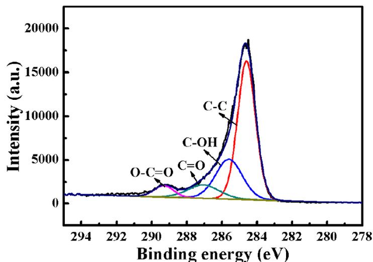
**Figure. S1.** The fitted high-resolution XPS spectrum of C 1s for the sample of NCNFs-1.
