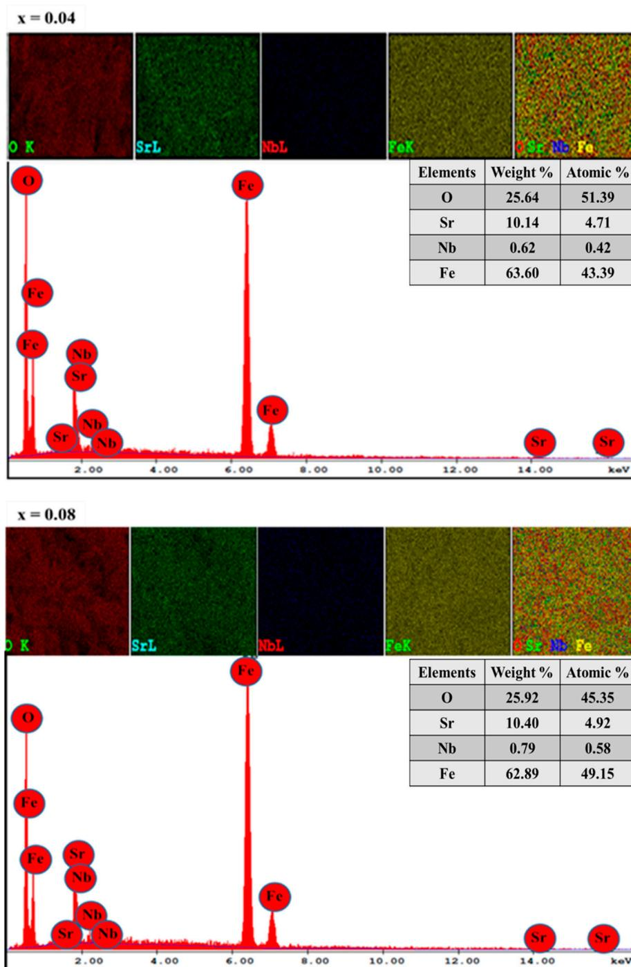
**Figure 3.** EDX patterns and elemental mapping results of  $\text{SrNb}_{0.04}\text{Fe}_{11.96}\text{O}_{19}$  and  $\text{SrNb}_{0.08}\text{Fe}_{11.92}\text{O}_{19}$  ( $0.00 \leq x \leq 0.08$ ) HFs.
