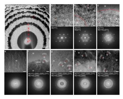
**Figure 5.** Crystal analysis of specimen. (**a**) TEM image of specimen. (**b**–**i**) HRTEM images (top) and corresponding SAED patterns (bottom) of these regions marked with red boxes in (**a**). Scale bar: 10 nm in (**b**–**i**).
