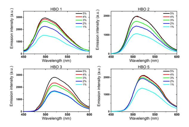
Figure S7.2 Comparison of emission profiles of 1-5% HBO dyes in PMMA matrix.
