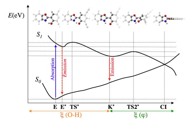
**Scheme S6.1.** Representation of the potential energy surface during the ESIPT process, with first a proton transfer (O-H reaction coordinate) and next a twist of the structure leading to a conical intersection (CI), back to the ground-state.
