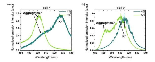
**Figure S7.1** Comparison of emission profile of 4% and 5% HBO **1** (a) and HBO **2** (b) in PMMA matrix. For HBO **1** blue-shifted emission from the aggregated form is visible, whereas for HBO **2** dual emission is observed.
