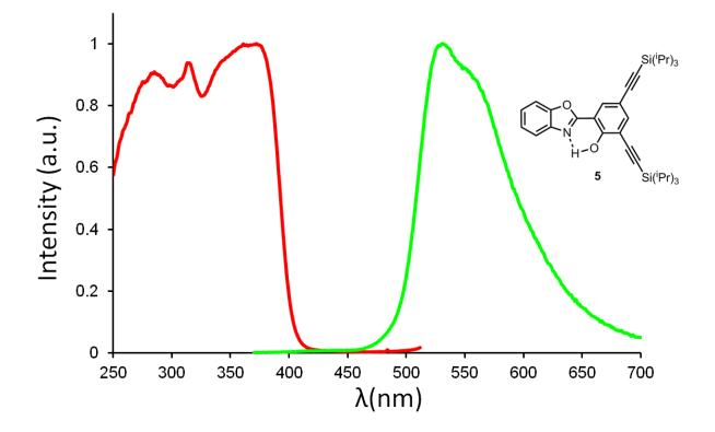
S5.3 Absorption, excitation and emission spectra of HBO dyes 1-5 in PMMA films
