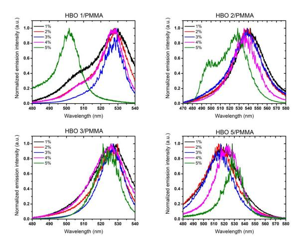
**Figure S7.4** Dependence of the light emission spectra on the doping concentration of ESIPT dyes 1-3 and 5 in the PMMA matrix.
