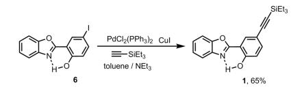
Scheme S1.1. Synthesis of HBO dye 1.
