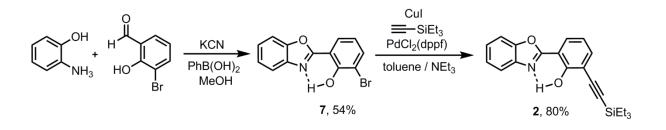
Scheme S1.2. Synthesis of HBO dye 2.
