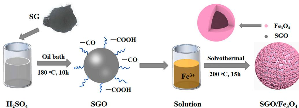
**Figure 1.** Preparation process of SGO/Fe<sub>3</sub>O<sub>4</sub> composites.
