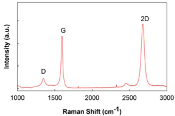
Figure S1. Raman spectrum of the graphene.
