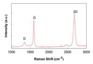
Figure S1. Raman spectrum of the graphene.
