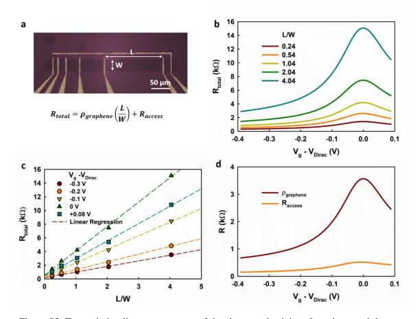
Figure S3. Transmission line measurement of the sheet conductivity of graphene and the access resistance. (a) The device for TLM study. (b) The transfer curves of each channel with different aspect ratios. (c) The linear regression analysis of the resistance measurement with respect to the aspect ratio. (d) The extracted sheet resistivity of graphene and the access resistance.
