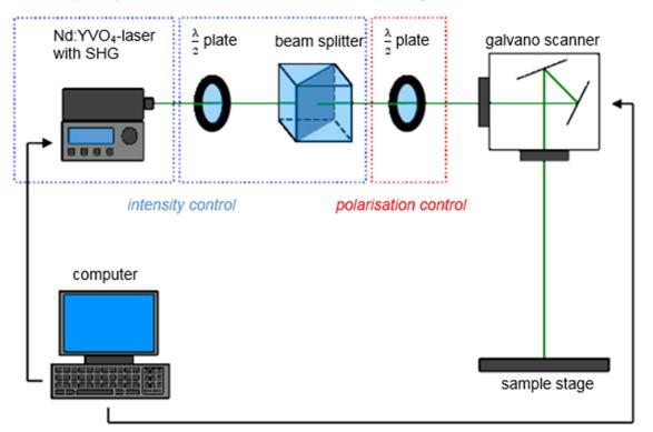
Following image shows the scheme of the used laser setup.
