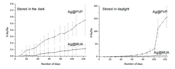
**Figure 2.** Change of sheet resistance over time of 32 nm diameter silver nanowires networks stored under atmospheric conditions in the dark (**left**) and in daylight (**right**).
