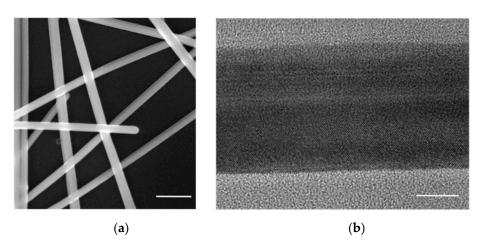
**Figure 1.** (a) SEM image of the MUA-coated network (scale bar: 100 nm). (b) ARM image of a passivated nanowire (scale bar: 10 nm).
