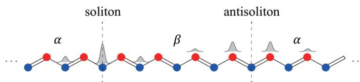
**Figure 3.** In a periodic system with two domain walls, a soliton-antisoliton pair must exist. Their site probability densities are shown. For a soliton (antisoliton), the probability density is finite on A (B) carbon atoms only.
