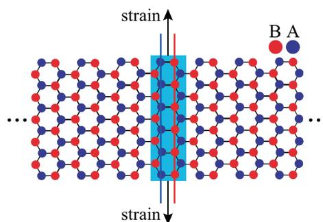
**Figure 6.** AGNR with local tensile strain applied perpendicular to ribbon direction in region  $D$  (blue area). A and B zigzag edge sites are shown on the blue and red lines.
