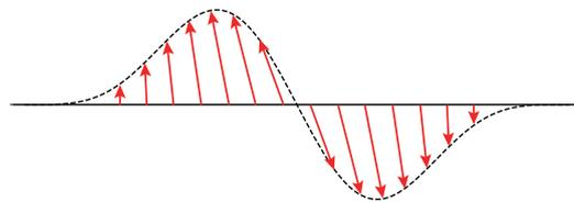
**Figure 7.** Domain-wall soliton corresponds to a topological kink. Pseudospin vector rotates by an angle of  $\pi$  out of the plane.
