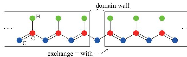
**Figure 2.** Two semi-infinite polyacetylene chains with a domain wall, which connects two different dimerized phases labeled  $-m$  and  $m$ . A double bond is shorter than a long bond and a Peierls lattice distortion is present. The directions of the double bonds vary in these two phases. Periodic boundary conditions cannot be imposed on this system as there is only one domain wall. Either a soliton or antisoliton is possible, but not both.
