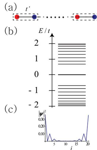
**Figure 4.** (a) Finite-length dimer chain with unit cell containing two carbon atoms connected by single bond. The Intra cell hopping  $t'$  is smaller than the inter cell hopping  $t$ . (b) Tight-binding energy spectrum. Two nearly degenerate gap states exist. (c) Probability density of gap state as function of site index  $i$ . A peak is apparent at the red (blue) site at the left (right) end. The probability densities of the bonding and antibonding states are almost identical.
