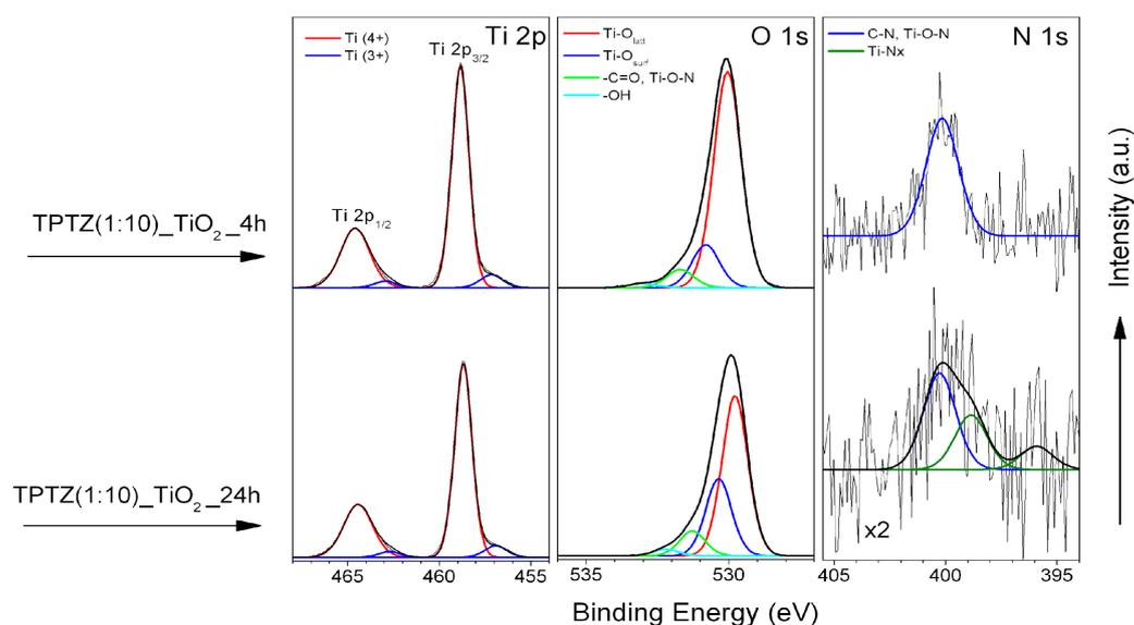
**Figure 8.** HR XPS spectra of Ti 2p, O 1s and N 1s for TPTZ(1:10)\_TiO<sub>2</sub> after various preparation time periods.
