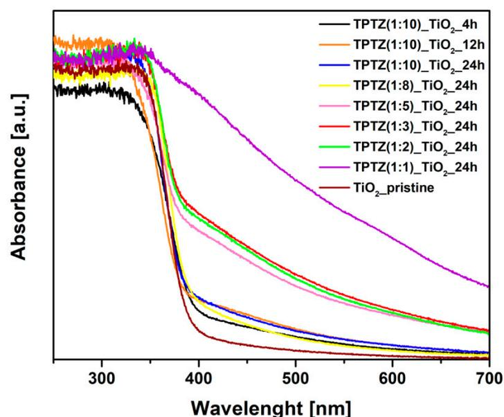
**Figure 6.** Time-dependent and IL content-dependent changes in the UV-VIS absorption of TPTZ\_TiO<sub>2</sub> microparticles.
