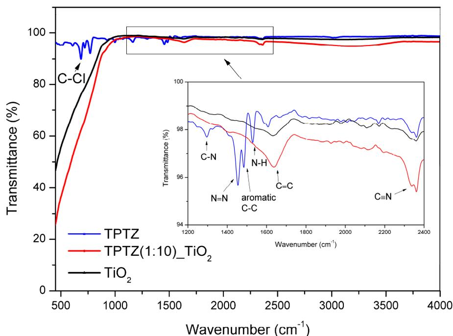
**Figure 9.** FTIR analysis of pristine IL and TPTZ(1:10)\_TiO<sub>2</sub>\_24 h sample in comparison with that of pristine TiO<sub>2</sub>.
