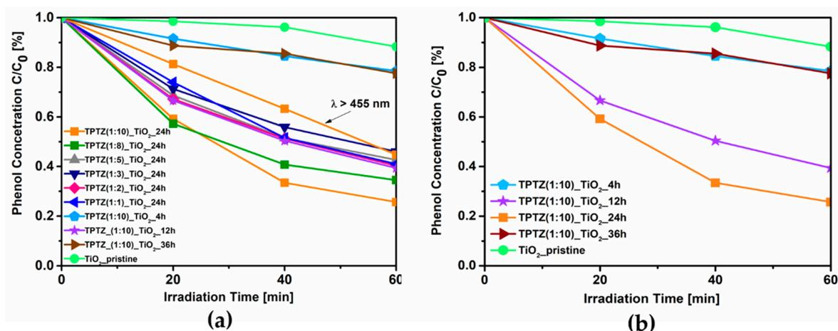
**Figure 2.** Efficiency of phenol degradation under visible irradiation ( $\lambda > 420$  nm or  $\lambda > 455$  nm) in the presence of the TPTZ\_TiO<sub>2</sub> samples prepared in various IL:TBOT molar ratios (a) and in different time periods (b).
