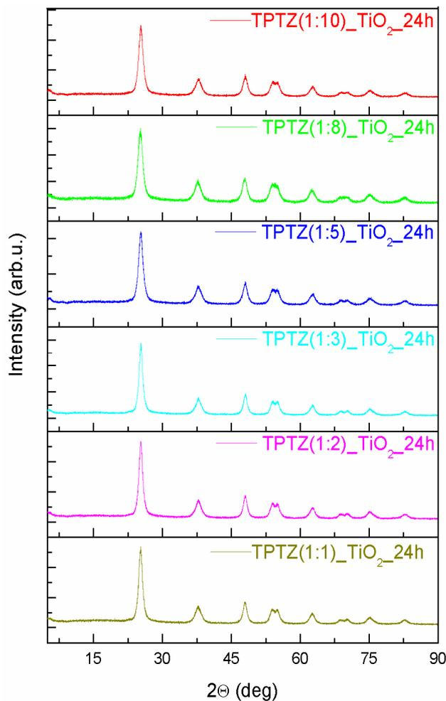
**Figure 3.** The XRD patterns of the  $\text{TiO}_2$  samples prepared by the ionic liquid (2,3,5-triphenyltetrazolium chloride)-assisted solvothermal method at variable IL contents (the IL:TBOT molar ratio ranged from 1:10 to 1:1).
