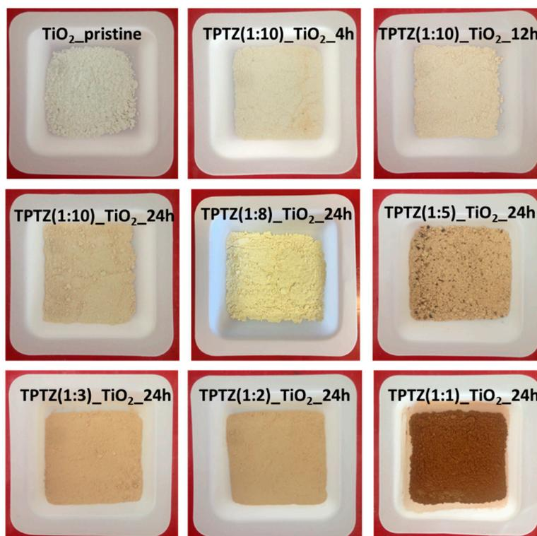
**Figure 7.** Colors of the samples of pristine  $\text{TiO}_2$  and  $\text{TiO}_2$  obtained using various molar ratios of  $[\text{TPTZ}][\text{Cl}]$  to TBOT in various times of the solvothermal process.
