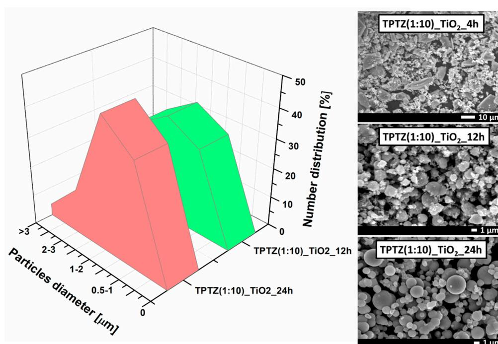
**Figure 5.** SEM images and particle size distribution of TiO<sub>2</sub> obtained by the solvothermal method in the presence of [TPTZ][Cl] ionic liquid after 4, 12 and 24 h.
