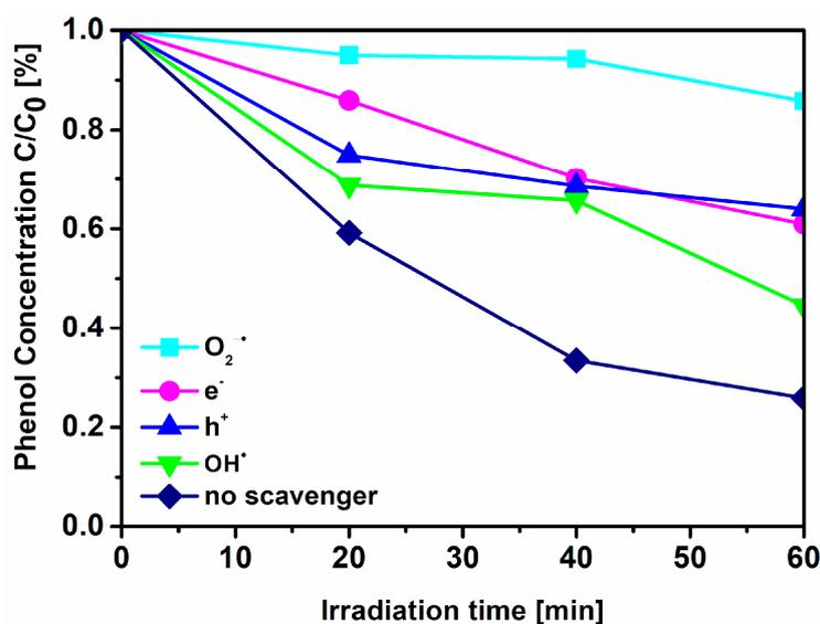
**Figure 10.** Effects of different scavengers on the effectiveness of phenol degradation under visible irradiation ( $\lambda > 420$  nm) in the presence of the TPTZ(1:10)\_TiO<sub>2</sub>\_24 h sample.
