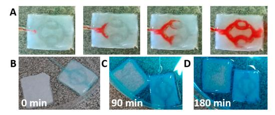
**Figure 5.** Perfusion and diffusion in the channeled hydrogel. (**A**) Fluid flow through the hydrogel channels. (**B**) Dye diffusion after 0 min, (**C**) after 90 min and (**D**) after 180 min in pristine-static and channeled-perfused samples.
