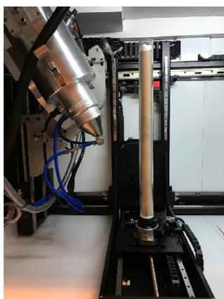
**Figure A1.** Inside view of micro computed tomography (micro-CT) scanner. On the left is the x-ray source. The sample is sitting on the rotating stage. After one sub scan, the sample will be moved one step up for another sub scan.
