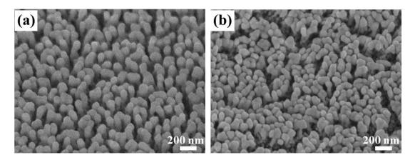
Figure S3. SEM images of (a) the non-leaning and (b) leaning Ag NPs.
