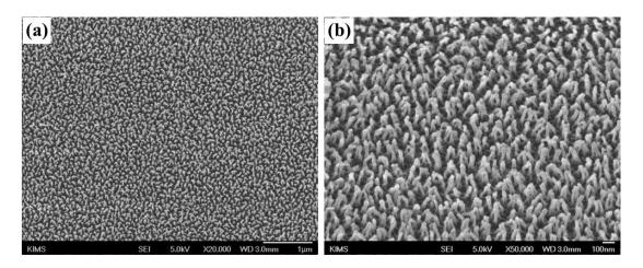
**Figure S1.** (a)–(b) FE-SEM images of the polyethylene terephthalate (PET) nanorods treated with an Ar plasma for 60 s.
