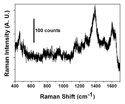
**Figure S6.** Raman spectrum obtained from the PDMS membrane. This spectrum was used to generate the red line in Figure 4a. A strong Raman shift related to the CH<sub>3</sub> vibrational bands appeared near 1400 cm<sup>-1</sup>.
