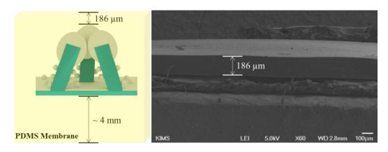
Figure S5. The SEM image indicated that the PDMS membrane was  $186~\mu m$  thick.
