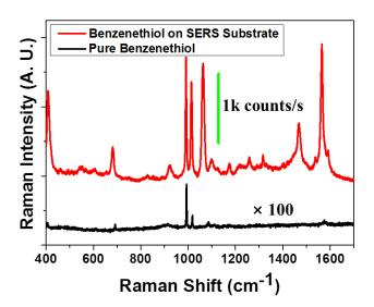
**Figure S4.** SERS spectrum measured from the benzenethiol monolayer-treated leaning Ag NPs (red line), and the normal Raman spectrum obtained from the pure benzenethiol solution (black line).
