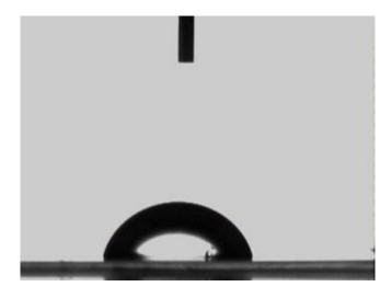
Figure S2. A water contact angle of 72° was obtained on the Ag/PET hybrid nanostructures.
