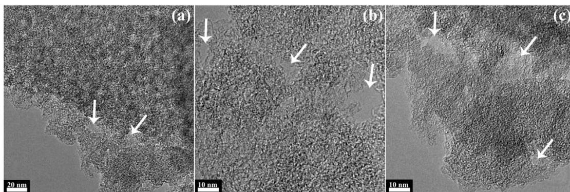
**Figure 3.** (a) Transmission electron microscopy (TEM) image of NPC with mesopores pointed by arrows at the edge. (b,c) High-resolution TEM images of the thin edges of NPC with mesopores pointed by arrows.
