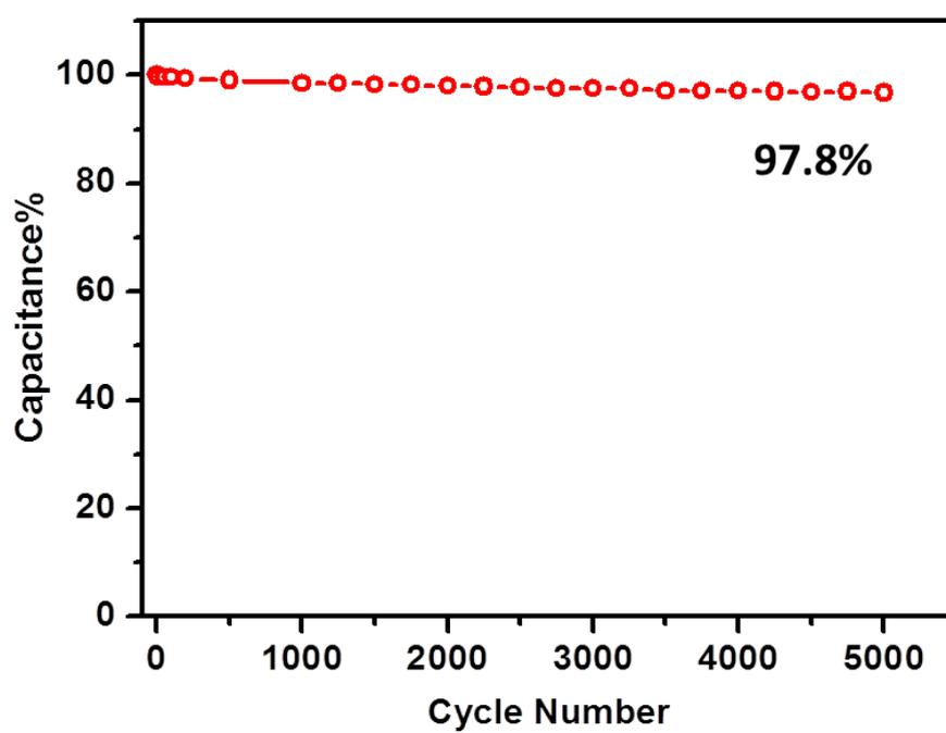
**Figure 4.** Specific capacitance retention for NPC at a current density of 10 A/g within 5000 cycles.
