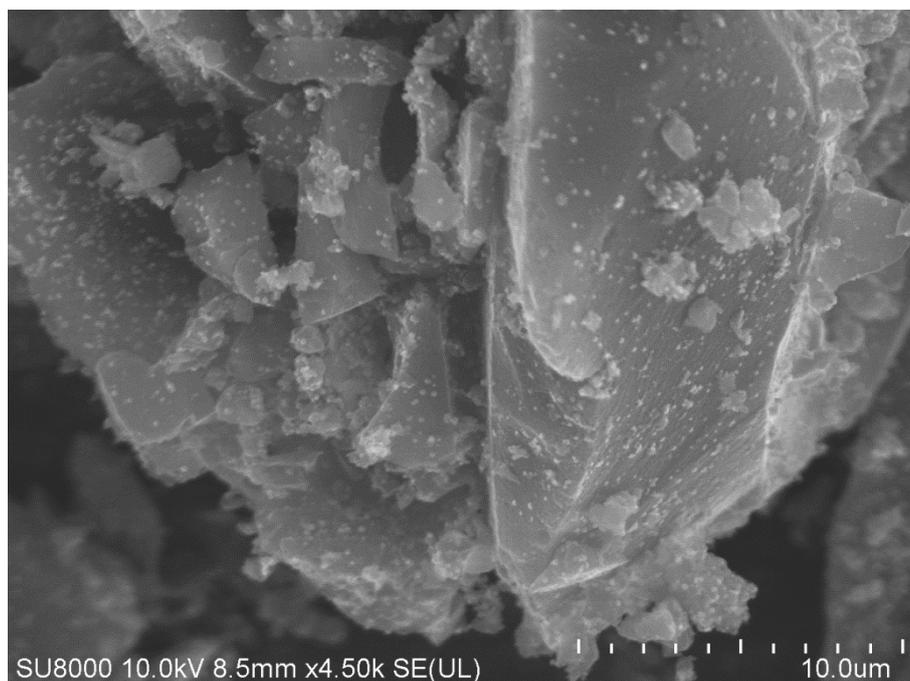
**Figure 2.** Scanning Electron Microscopy (SEM) image of nanoporous carbon (NPC).
