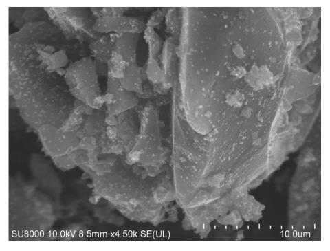
Figure 2. Scanning Electron Microscopy (SEM) image of nanoporous carbon (NPC).
