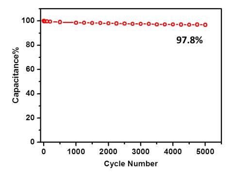
Figure 4. Specific capacitance retention for NPC at a current density of 10 A/g within 5000 cycles.
