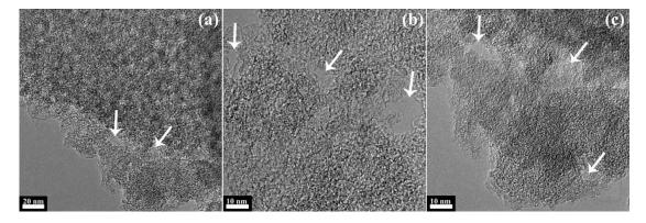
**Figure 3.** (a) Transmission electron microscopy (TEM) image of NPC with mesopores pointed by arrows at the edge. (b,c) High-resolution TEM images of the thin edges of NPC with mesopores pointed by arrows.
