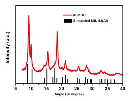
**Figure 1.** X-ray diffraction (XRD) pattern of Al-based metal-organic complex (Al-MOC) and the peak position of simulated MIL-53 (Al).
