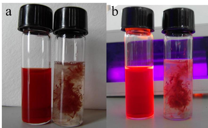
Fig. S1. Optical photos of both the MEA-CdTe NCs dispersion (the left bottle) and the CdTe/SA blend (the right bottle) under (a) daylight and (b) UV-light.
