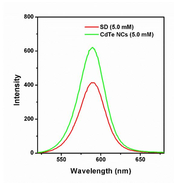
Fig. S3. PL spectra of ThGA-CdTe NCs dispersion and ThGA-CdTe/SA SD with the same NCs' concentration after been stored for 30 days.
