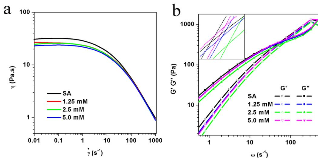
Fig. S4. Rheological properties of SDs and the 4wt% SA solution at 50 °C: (a) shearing rate ( $\dot{\gamma}$ ) dependence of viscosity ( $\eta$ ); (b) angular frequency dependence ( $\omega$ ) of storage modulus ( $G'$ ) and loss modulus ( $G''$ ). Inset: the magnification of the intersection of  $G'$  and  $G''$ .
