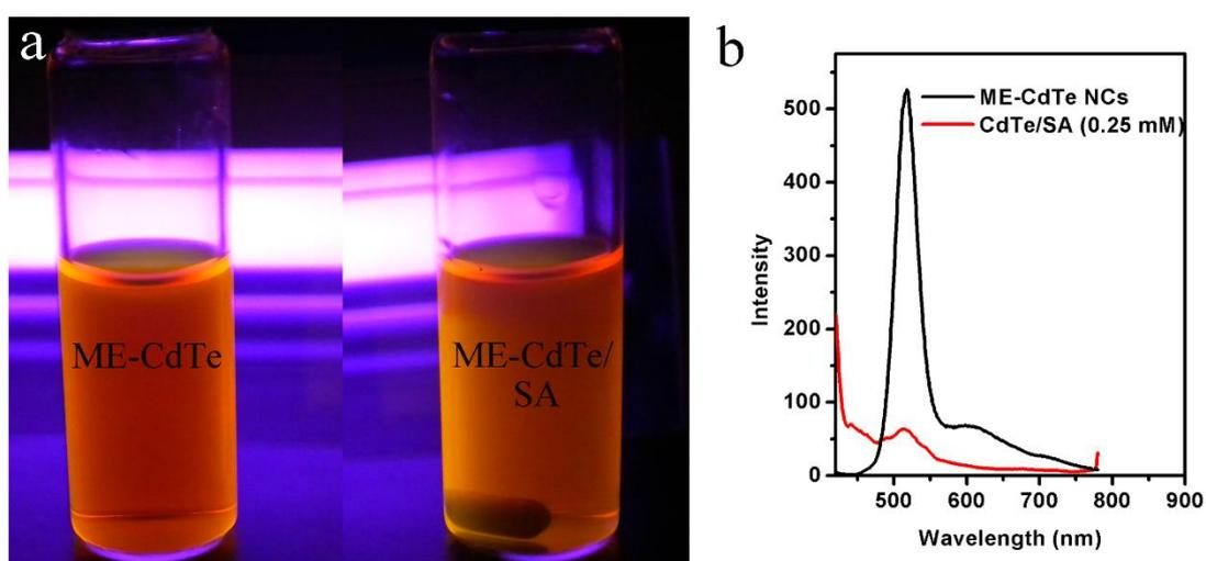
Fig. S2. (a) Optical photos of the ME-CdTe NCs dispersion and the ME-CdTe/SA blend (in which the ME-CdTe concentration is 0.25 mM) under UV-light. (b) PL spectra of the ME-CdTe NCs dispersion and the ME-CdTe/SA blend after stored in the dark for 30 days.
