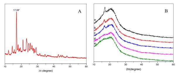
**Figure 3.** XRD spectra of Cur (**A**). XRD spectra of PLA/PEG/Cur CNFs with the different weight ratio (PEG:PLA): (**a**) 1:1; (**b**) 1:3; (**c**) 1:5; (**d**) 1:7; (**e**) 1:9 (**B**).
