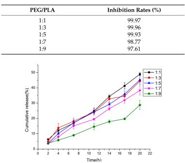
**Figure 8.** Initial burst release of Cur from PLA/PEG/Cur CNFMs with different weight ratios (PEG:PLA).
