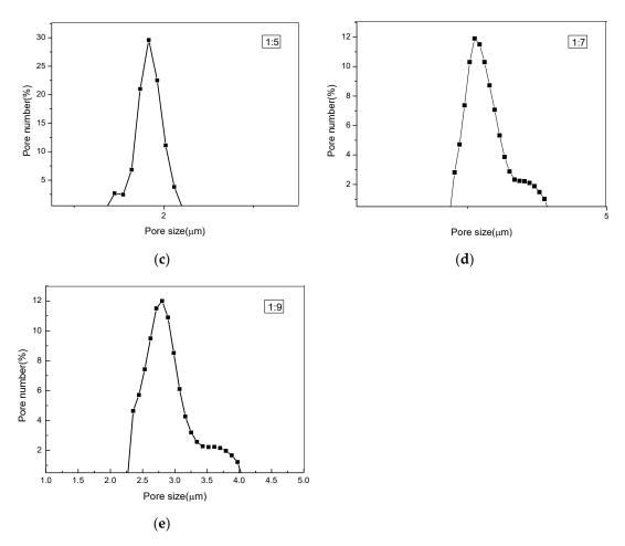
**Figure 4.** The pore size distributions of PLA/PEG/Cur nonporous composite nanofiber membranes (CNFMs) with different weight ratios (PEG:PLA): (**a**) 1:1; (**b**) 1:3; (**c**) 1:5; (**d**) 1:7; (**e**) 1:9.
