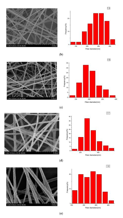
**Figure 1.** SEM pictures of the electrospun polylactide/polyethylene glycol/curcumin (PLA/PEG/Cur) carbon nanofibers (CNFs) with different weight ratios (PEG:PLA). The right figures were the according diameter distribution: (**a**) 1:1, (**b**) 1:3, (**c**) 1:5, (**d**) 1:7, (**e**) 1:9.
