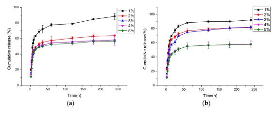
**Figure 5.** Cumulative release of Cur from porous and nonporous PLA/PEG/Cur CNFs with the different Cur contents: (**a**) Nonporous CNFs; (**b**) Porous CNFs.
