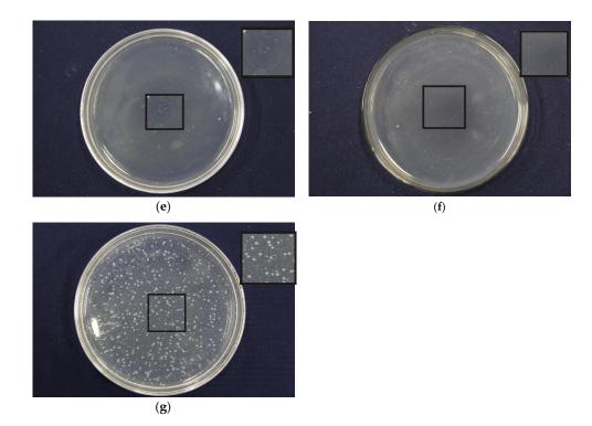
**Figure 7.** Effects of different composite ratio on antibacterial properties of PLA/PEG/Cur nanofibers membranes: (a) PEG:PLA = 1:7 (0% Cur); (b) PEG:PLA = 1:1 (3% Cur); (c) PEG:PLA = 1:3 (3% Cur); (d) PEG:PLA = 1:5 (3% Cur); (e) PEG:PLA = 1:7 (3% Cur); (f) PEG/PLA = 1:9 (3% Cur); (g) cotton.
