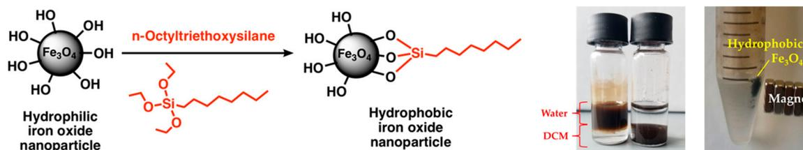
**Figure 3.** Surface functionalization of iron oxide nanoparticles using n-octyltriethoxysilane. (First photograph) Hydrophobic magnetite nanoparticles (NPs) phase separate into organic medium. Left: hydrophilic nanoparticles. Right: hydrophobic nanoparticles. (Second photograph) Hydrophobic  $\text{Fe}_3\text{O}_4$  attracted by a set of magnets.
