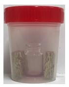
**Figure S10**. Left (different board pieces, from left to right PB 27 mm, PB 10 mm, PB 16 mm, FB 35 mm). Right (system for the detection of the formaldehyde emission from board pieces).
