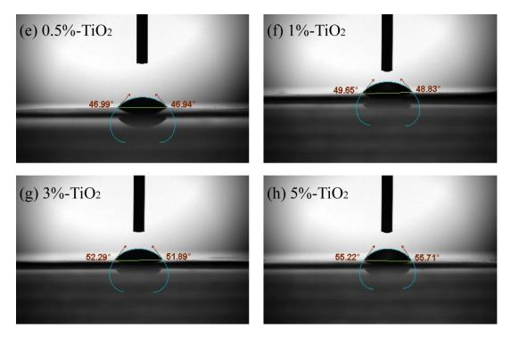
Figure S1. The contact angles for the various blend films: (a) 0. 5%-MMT, (b) 1%-MMT, (c) 3%-MMT, (d) 5%-MMT, (e) 0. 5%-TiO<sub>2</sub>, (f) 1%-TiO<sub>2</sub>, (g) 3%-TiO<sub>2</sub>, (h) 5%-TiO<sub>2</sub>.
