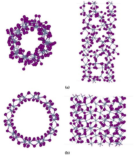
**Figure S1.** Snapshots of MD at 5 ps with top and side views at 300 K for (**a**) (5,0)-ZZ NT (**b**) (5,5)-AC NT.
