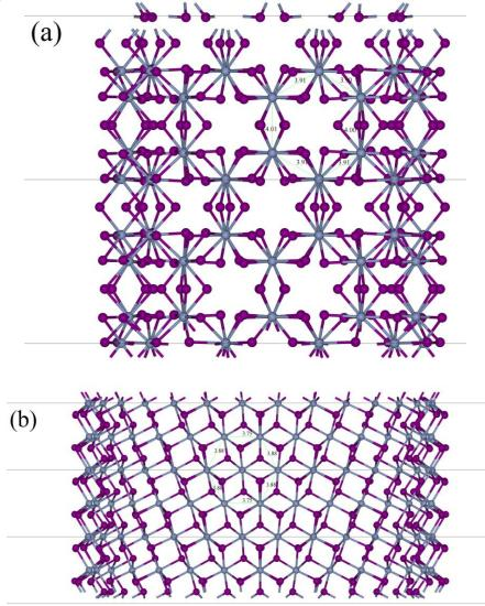
**Figure S2.** Atomic structure of chromium(III) iodide (CrI<sub>3</sub>) NTs: (**a**) illustration of (10,0)-ZZ NT (**b**) (10,10)-AC NT with side views.
