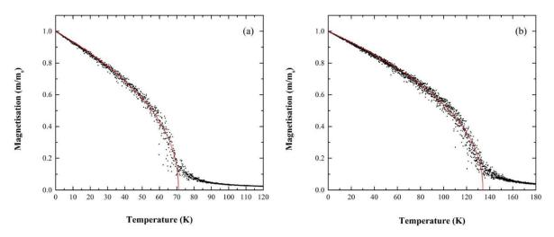
Figure S4. Temperature dependent magnetization curve for CrI<sub>3</sub>(a) (7,0)-ZZ NT, and (b) (12,0)-ZZ NT.
