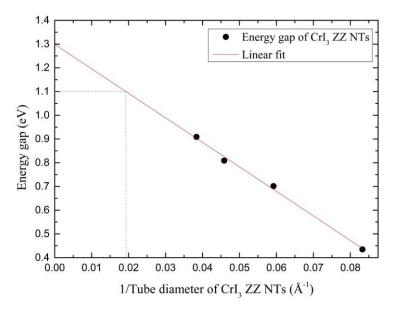
Figure S3. The energy gap of CrI<sub>3</sub> ZZ NTs with respect to diameter reciprocals.
