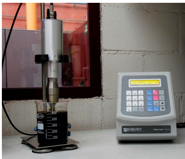
Figure 3. Sonicator 750 W used to produce the DNF.
