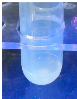
Figure 8. The photograph of the colloidal PNC solution produced by an excessive amount of OAm after storage in air for five days under the UV irradiation. This indicates that CsPbBr 3 PNCs are very unstable when the amount of OAm is excessive.
