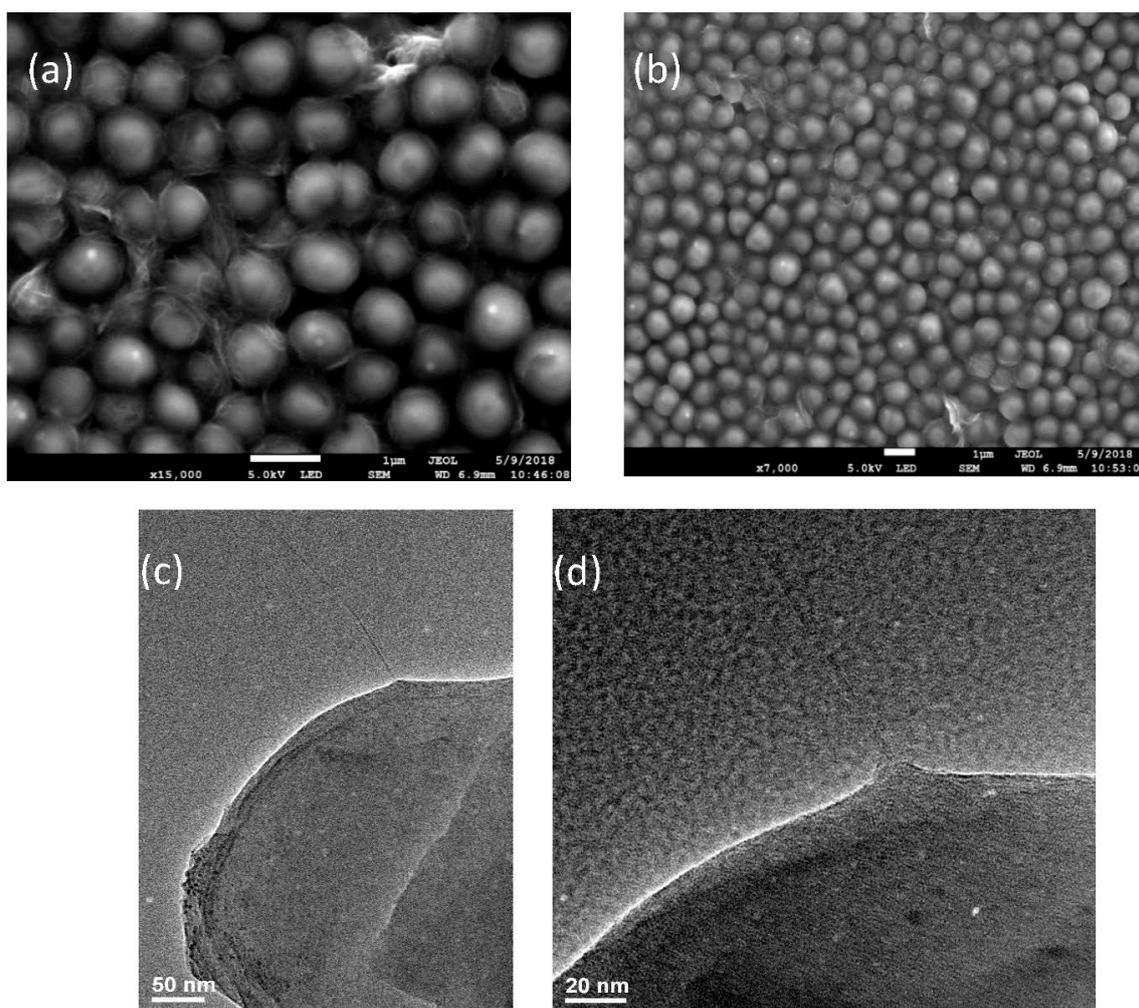
**Figure 7.** Electron Microscopy (a,b) Scanning electron microscopy (SEM) images of bacterial cells subject to SWCNT/methicillin hybrids, (c,d) Transmission electron microscopy (TEM) images of SWCNTs penetrating bacterial cell wall in cultures subject to SWCNT/methicillin.
