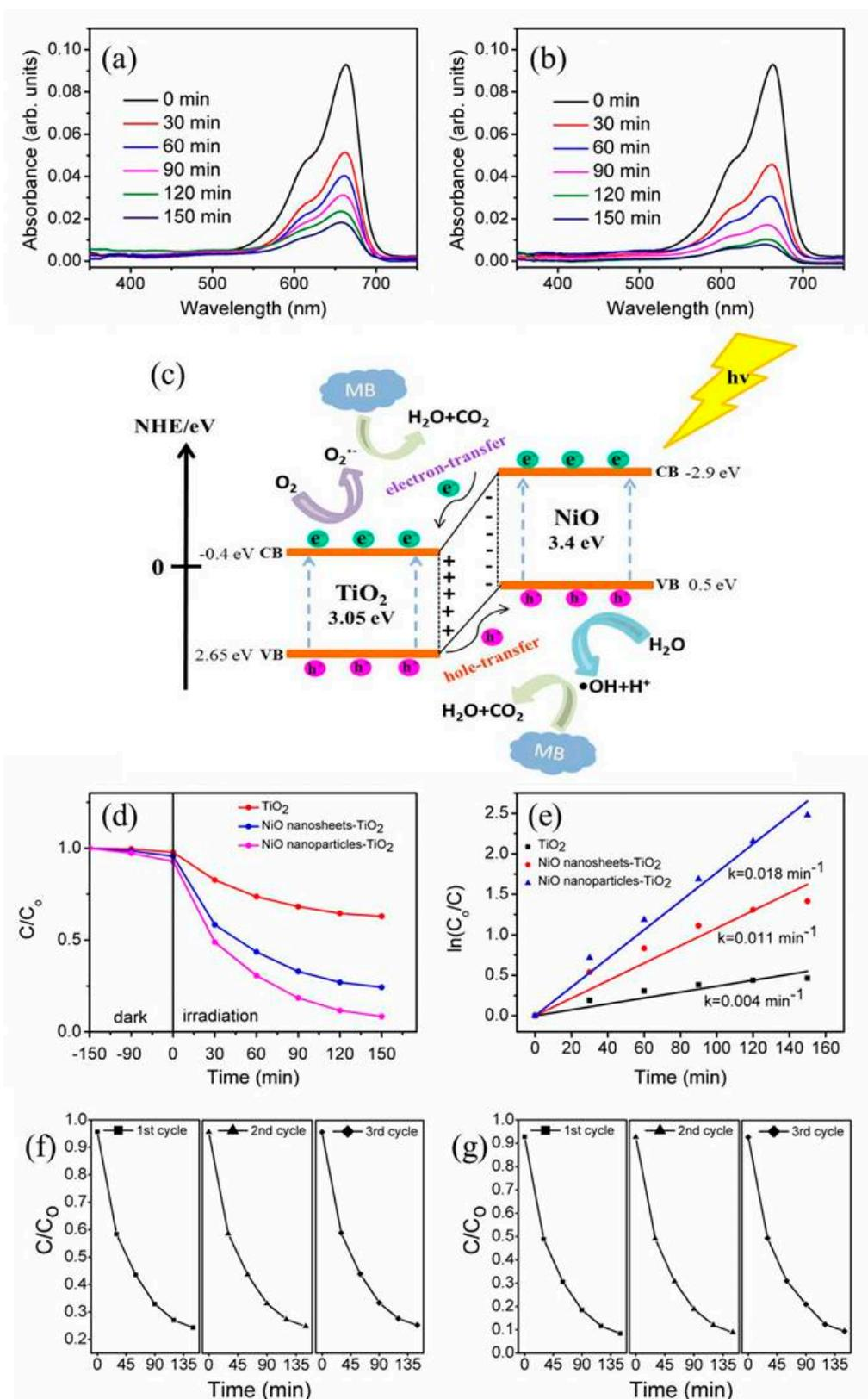
**Figure 6.** Intensity variation of absorbance spectra of the methylene blue (MB) solution vs. irradiation duration containing various TiO<sub>2</sub>-NiO composites under solar light irradiation: (a) NST. (b) NPT. (c) Schematic of photodegradation process of TiO<sub>2</sub>-NiO composites toward MB. (d) The ratio of the
