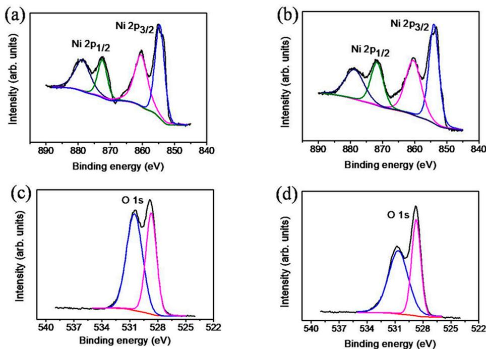
**Figure 4.** High-resolution XPS spectra in Ni 2p region of TiO<sub>2</sub>-NiO composites formed at various temperatures: (a) 350 °C and (b) 500 °C. High-resolution XPS spectra in O 1s region of TiO<sub>2</sub>-NiO composites formed at various temperatures: (c) 350 °C and (d) 500 °C.
