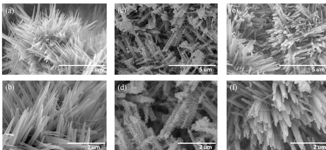
**Figure 1.** (a,b) Low- and high-magnification SEM images of TiO<sub>2</sub> nanostructures. (c,d) Low- and high-magnification SEM images of TiO<sub>2</sub>-NiO composites formed at 350 °C. (e,f) Low- and high-magnification SEM images of TiO<sub>2</sub>-NiO composites formed at 500 °C.
