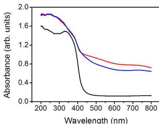
**Figure 5.** Optical absorbance spectra of the pristine TiO<sub>2</sub> (black), NST (blue), and NPT (red).
