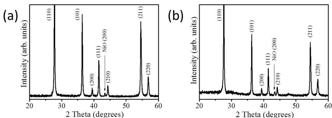
**Figure 2.** XRD patterns of TiO<sub>2</sub>-NiO composites formed at (a) 350 °C and (b) 500 °C. The arrow represents the position of NiO Bragg reflection.
