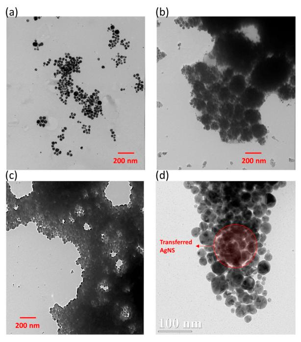
**Figure 2.** TEM images of AgNCs and AgNSs before/after phase transfer. (**a**): AgNCs, (**b**): AgNSs before phase transfer, (**c**): Transferred AgNSs, (**d**): Transferred AgNSs with high resolution).
