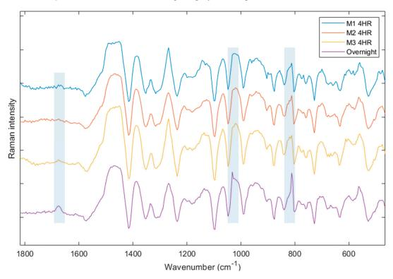
**Figure 7.** SERS spectra of MeSA VOCs according to the collection times. M1 4HR: Mixture with 1 mg of polymer for 4 h, M2 4HR: Mixture with 2 of mg polymer for 4 h, M3 4HR: Mixture with 3 mg of polymer for 4 h, overnight: Averaged over three concentrations overnight. MeSA standard Raman spectrum is available in the Supplementary Materials, Figure S1.
