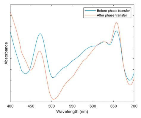
Figure 5. UV/Vis absorption spectrum of AgNSs before/after phase transfer.
