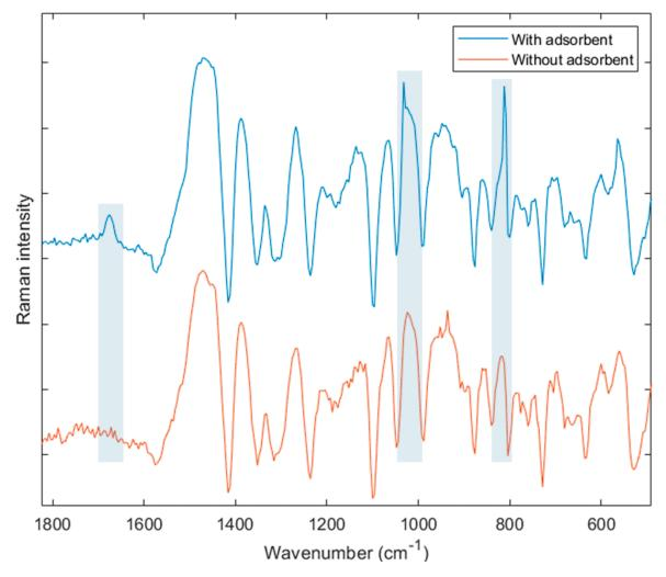
**Figure 8.** The effect of adsorbent on SERS spectra of MeSA VOC. MeSA standard Raman spectrum is available in the Supplementary Materials, Figure S1.
