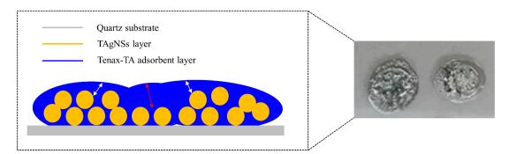
Figure 6. Scheme of transferred AgNSs-polymer complex-based SERS substrate.
