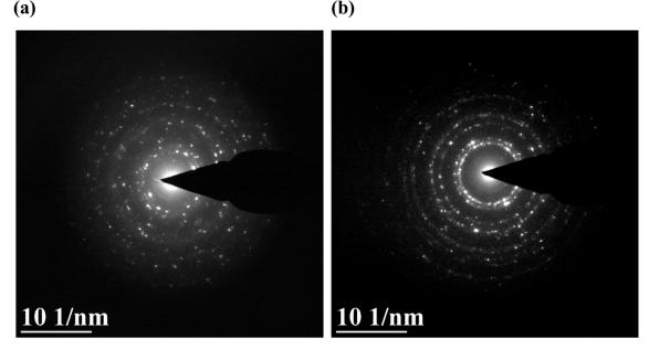
Figure 4. Crystal diffraction pattern of AgNSs (a) before phase transfer and (b) after phase transfer.
