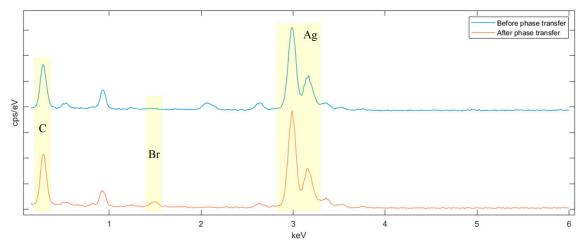
Figure 3. EDX spectra of AgNSs before/after phase transfer.
