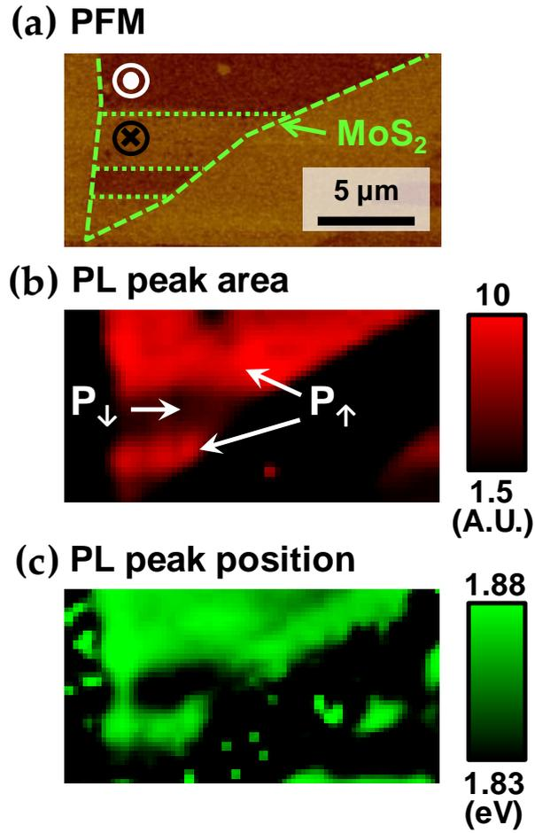
**Figure S3. Microscale PL modulation of the ML-MoS<sub>2</sub> driven by the domain-engineered BFO thin film.** (a) PFM image of the ML-MoS<sub>2</sub> on a BFO thin film poled in the stripe pattern. The bright and dark areas indicate the regions in the P<sub>↑</sub> and P<sub>↓</sub> states, respectively, and were achieved by applying  $V_P$  of  $\pm 12$  V. Maps of (b) PL peak area (c) PL peak position of the identical ML-MoS<sub>2</sub> in (a) scanned after poling process.
