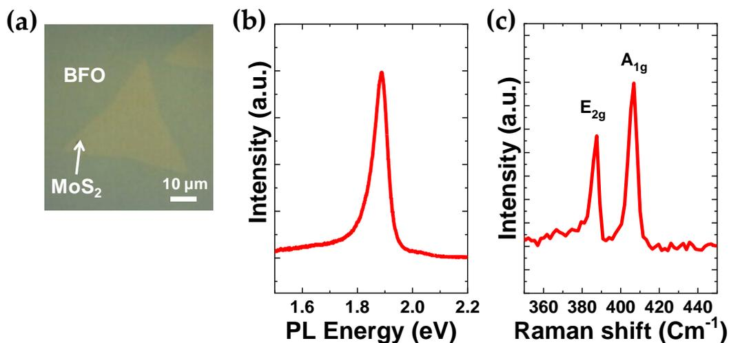
**Figure S1. Optical characterization of the ML-MoS<sub>2</sub>/BFO heterostructure.** (a) Optical microscopy image of a representative ML-MoS<sub>2</sub> flake wet-transferred on a BFO thin film surface. (b) PL and (c) Raman spectra measured from the ML-MoS<sub>2</sub> flake in (a).
