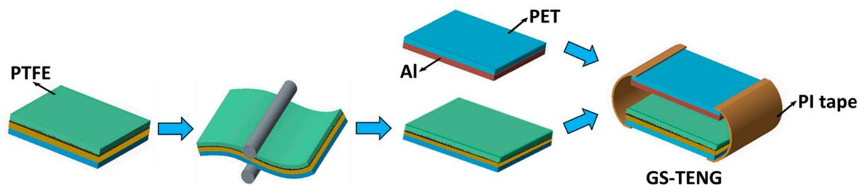
**Figure 2.** Schematic illustration of the fabrication process of the graphite-coated sandpaper-based triboelectric nanogenerator (GS-TENG).
