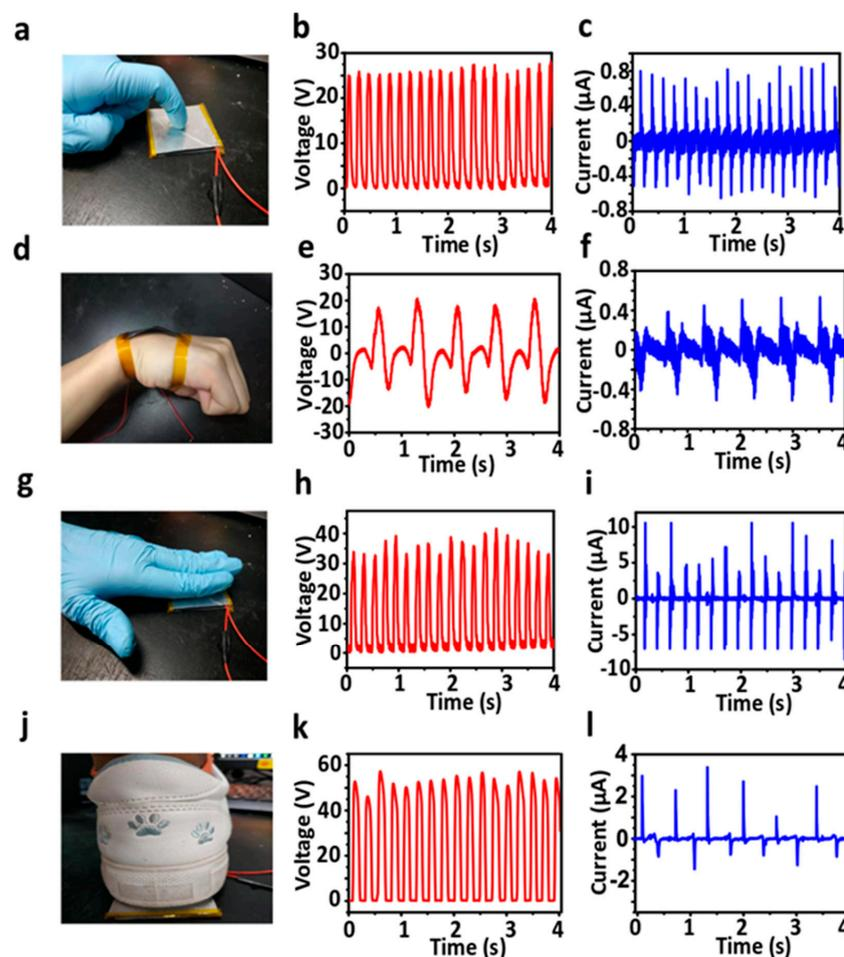
**Figure 7.** Investigation of energy harvesting from human body movements as an active biomechanical sensor. Optical image of harnessing biomechanical movement and corresponding open-circuit voltage ( $V_{oc}$ ) and short-circuit current ( $I_{sc}$ ) on GS-TENG (a–c) finger touch, (d–f) wrist movement, (g–i) hand tap and (j–l) foot stamping respectively.
