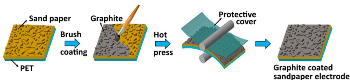
**Figure 1.** Schematic of the complete fabrication process of the graphite-coated sandpaper electrode.
