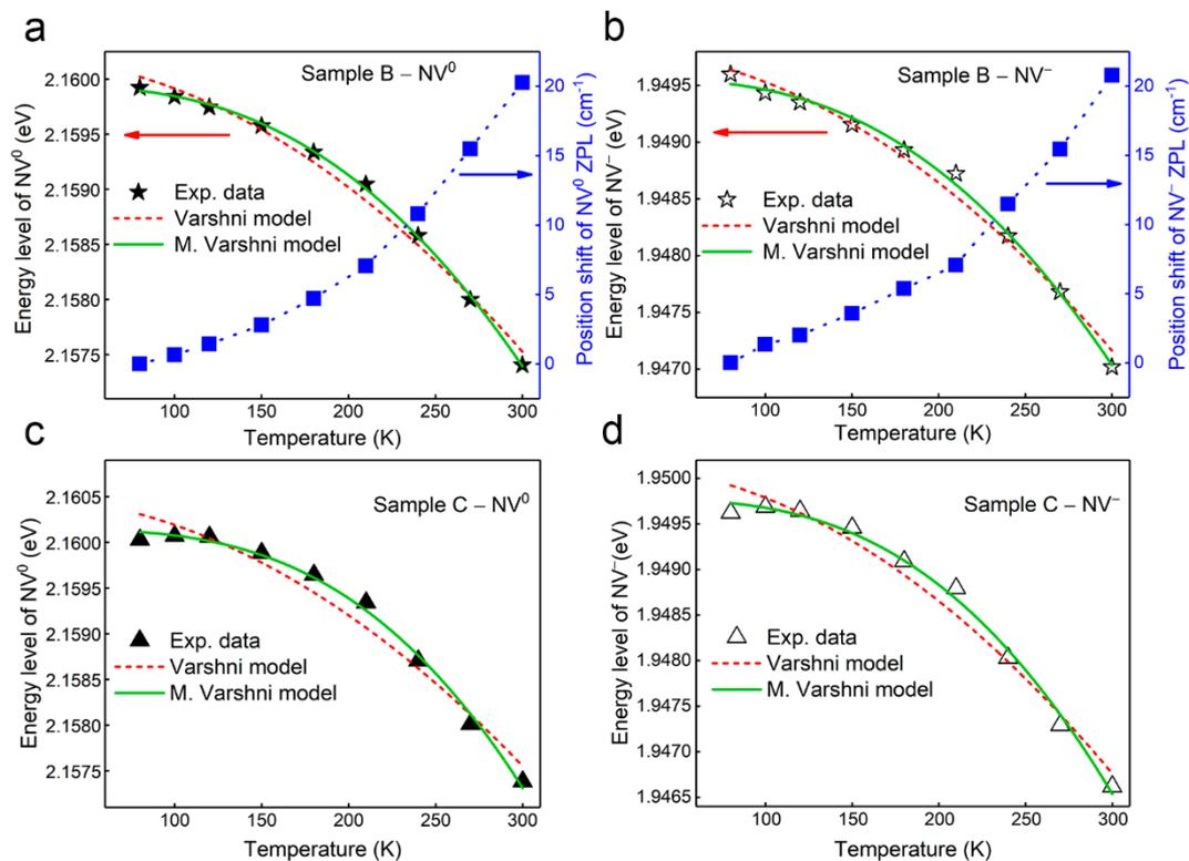
**Figure 3.** The ZPL position and energy level variation of (a)  $NV^0$  and (b)  $NV^-$  centers with temperature for diamond sample Sample B; the energy level variation of (c)  $NV^0$  and (d)  $NV^-$  centers with temperature for diamond sample Sample C.
