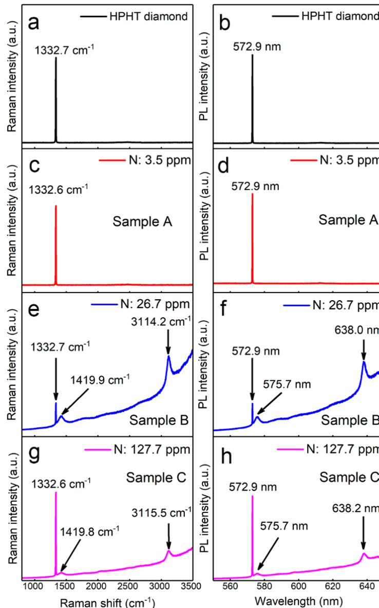
**Figure 1.** Raman and photoluminescence (PL) spectra of diamond samples in room temperature: (a,b) high pressure high temperature (HPHT) diamond and epitaxial chemical vapor deposition (CVD) diamond with nitrogen concentrations of (c,d) 3.5 ppm, (e,f) 26.7 ppm and (g,h) 127.7 ppm.
