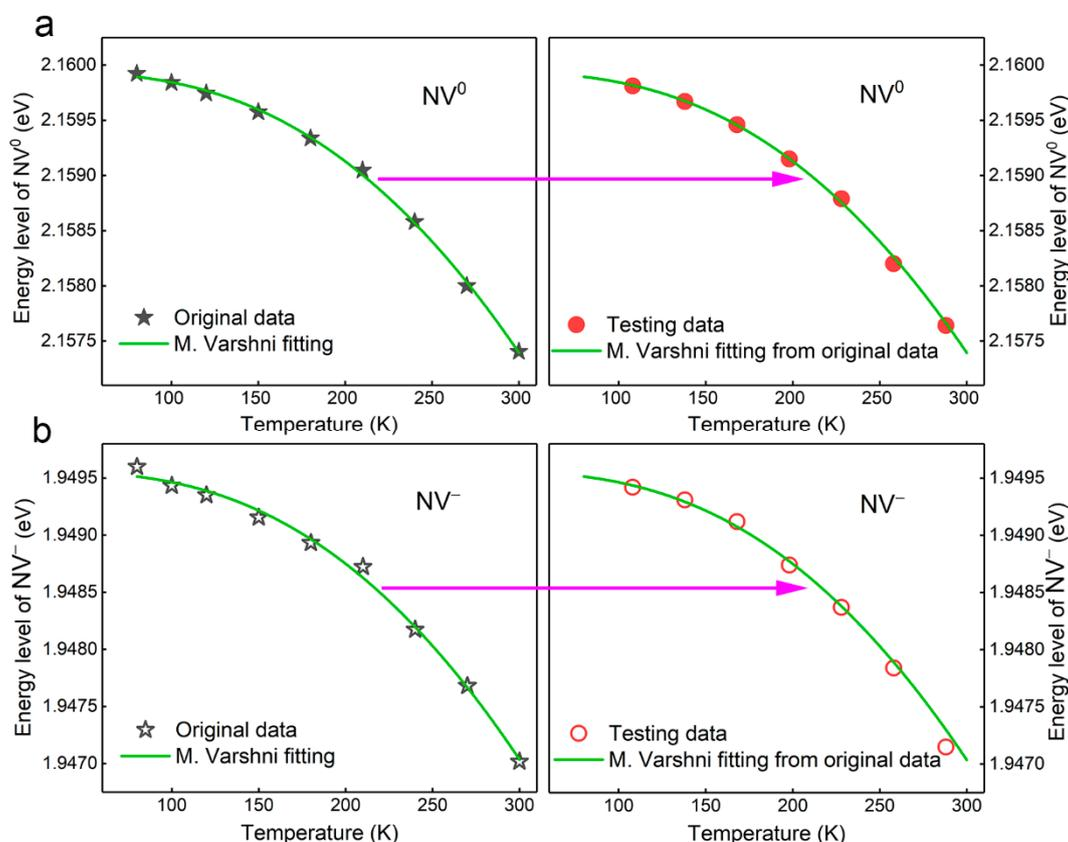
**Figure 4.** The accuracy determination of (a)  $NV^0$  and (b)  $NV^-$  centers in temperature measurement based on the energy level shifts.
