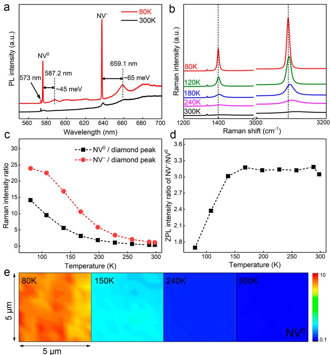
**Figure 2.** (a) PL spectra and (b) Raman spectra of the diamond sample with temperature measured from 80 K to 300 K. The zero-phonon line (ZPL) intensity ratio of nitrogen-vacancy (NV) centers to (c) the diamond first-order Raman phonon line, (d) the ZPL intensity ratio of  $NV^-$  to  $NV^0$  from 80 K to 300 K, and (e) Raman mapping of the ratio of the ZPL intensity of the  $NV^0$  center to diamond peak with a size of about 5  $\mu m$   $\times$  5  $\mu m$ .
