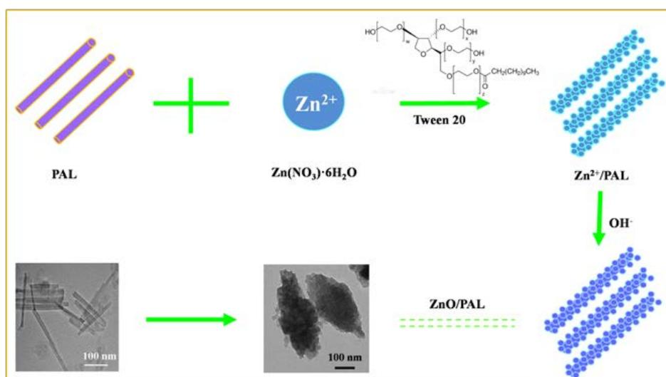
**Figure 5.** Schematic illustration for the preparation of spindle-like ZnO/PAL.
