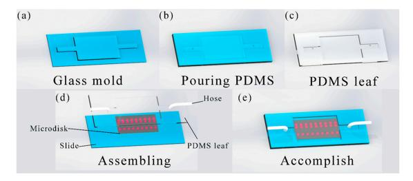
Figure 2. 3-D schematic diagram shows the fabrication process of the optofluidic microdisk device.
