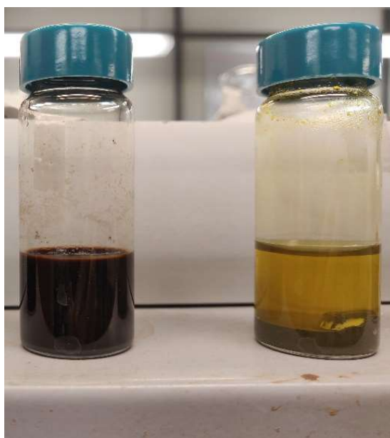
Figure S3. Sedimentation test evaluating stability of the nanoink.
