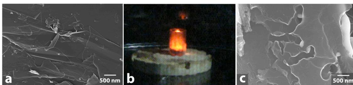
**Figure 11.** Effect of microwave irradiation on mixture of graphite and metal-containing compounds: initial graphite surface (a); microwave heating of mixture of graphite and metal compound (b); graphite surface with traces of etching by particles of silver (c).
