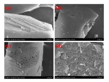
**Figure 1.** Scanning electron microscope (SEM) images of the NPC-500 (**a**); HPC-600 (**b**); HPC-700 (**c**); and HPC-800 (**d**).
