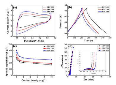
**Figure 6.** Electrochemical performance of all the HPC electrodes measured in a three-electrode system: (a) Cyclic voltammetry (CV) curves at a scan rate of 10 mV·s<sup>-1</sup>; (b) Galvanostatic charge/discharge (GCD) curves at a current density of  $1 \text{ A} \cdot \text{g}^{-1}$ ; (c) specific capacitances at different current densities; and (d) Nyquist plots and inset magnified image.
