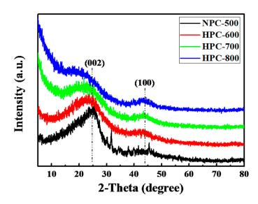
Figure 2. X-ray Diffraction (XRD) patterns of the NPC-500, HPC-600, HPC-700, and HPC-800.
