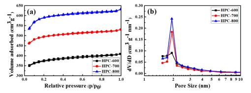
**Figure 4.** N<sub>2</sub> adsorption isotherms (**a**) and Barrett–Joyner–Halenda (BJH) pore size distributions (**b**) for the HPCs.
