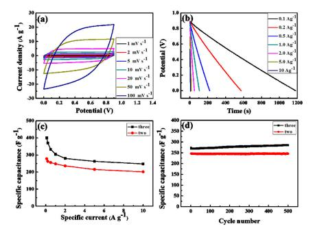
**Figure 7.** Electrochemical performance of the HPC-800 electrode measured in a two-electrode system: (a) CV curves at different various scan rates; (b) GCD curves under different current densities; (c) capacity profiles at different current densities; (d) the long cycle life over 500 cycles at a current density of  $1 \text{ A} \cdot \text{g}^{-1}$ .
