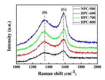
Figure 3. Raman spectra of the NPC-500, HPC-600, HPC-700, and HPC-800.
