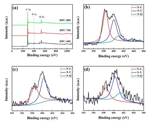
**Figure 5.** X-ray photoelectron spectroscopy (XPS) survey spectra (**a**); N 1s spectra of the HPC-600 (**b**); HPC-700 (**c**); and HPC-800 (**d**).
