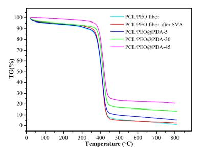
**Figure 3.** Thermogravimetry (TG) curves of the prepared PCL/PEO electrospun fibers before and after SVA treatment and the PCL/PEO@PDA composites of different PDA modification intervals (5 h, 30 h, and 45 h).
