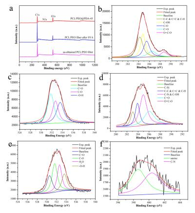
**Figure 4.** Survey XPS spectra of the fiber composites (**a**) and the peak deconvolutions: (**b**,**c**), C1s and O1s in the PCL/PEO fiber after SVA treatment, respectively; (**d**–**f**), C1s, O1s, and N1s in the PCL/PEO@PDA-45 composite, respectively.
