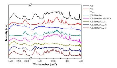
Figure 5. FT-IR spectra of the initial materials and the obtained composite fibers.
