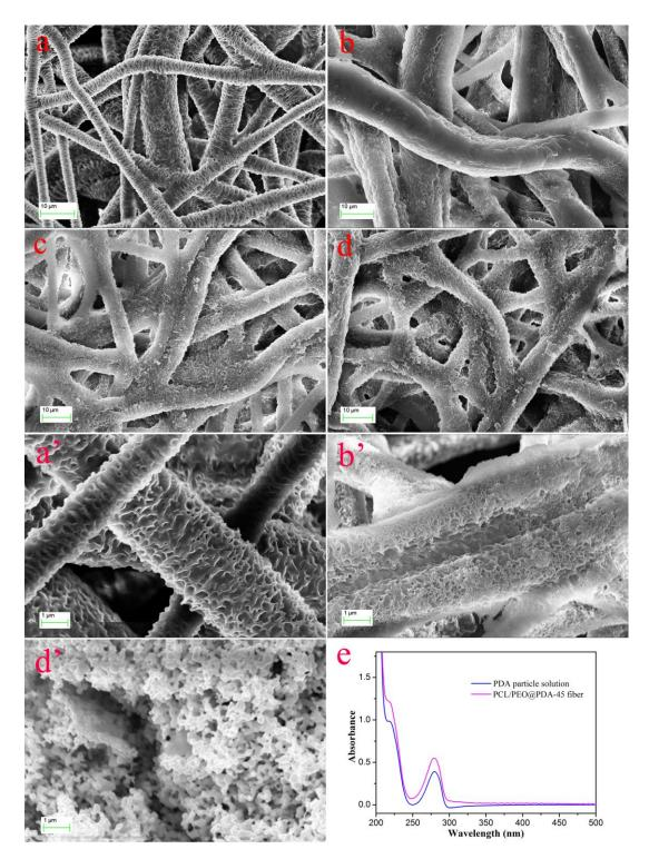
**Figure 2.** SEM images of the solvent vapor annealing (SVA)-treated PCL/PEO fibers (**a**,**a**') and PCL/PEO@PDA of different modification time intervals (**b**,**b**'), 5 h; (**c**), 30 h; (**d**,**d**'), 45 h; (**e**) UV-vis spectra of the PDA solution and PCL/PEO@PDA-45 fiber composite.
