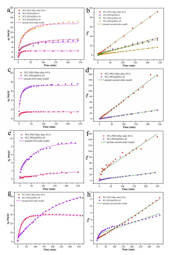
**Figure 6.** Adsorption kinetics curves of the prepared composite fibers on methylene blue (MB) (**a**,**b**), Rhodamine B (RhB) (**c**,**d**), Safranine T (ST) (**e**,**f**), and methyl orange (MO) (**g**,**h**) at 298 K.
