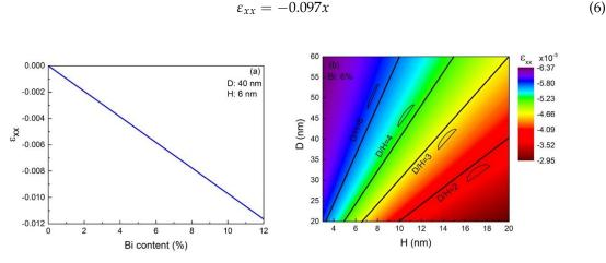
**Figure 2.** (a) The simulated average in-plane strain  $\varepsilon_{xx}$  in the InPBi QDs versus the Bi content with fixed diameter and height of the QDs of 40 nm and 6 nm, respectively; (b) contour map of the average  $\varepsilon_{xx}$  versus the diameter and height of the InPBi QDs with the Bi content of 6%. The black lines represent the aspect ratio of 2, 3, 4 and 6, respectively, with the diagrammatic sketch of the shape of the QD next to each line.
