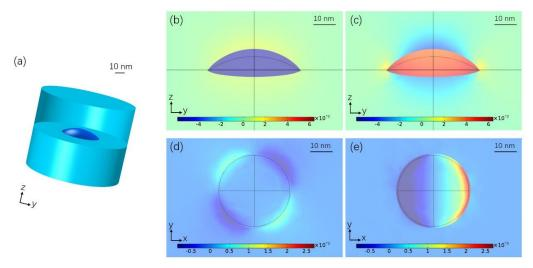
**Figure 1.** (a) Three-dimensional schematic of the proposed InPBi QD structure. The strain distribution of (b)  $\varepsilon_{xx}$  and (c)  $\varepsilon_{zz}$  in the yz plane; (d)  $\varepsilon_{xy}$  and (e)  $\varepsilon_{xz}$  in the xy plane for the InPBi QDs in InP with Bi content of 6%, diameter of 40 nm and height of 6 nm. The deformation is exaggerated by 100 times.
