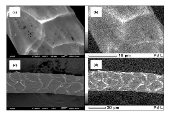
**Figure 1.** Images of the palladium–merino wool nanocatalysts prepared from a 260 mg L<sup>-1</sup> Pd<sup>2+</sup> solution at 100 °C and pH: 3.0 (S1) were taken by (**a**) Backscatter SEM; (**b**) Energy Dispersive X-ray Analysis (EDS) elemental maps for Pd (white dots); (**c**) Backscatter SEM; (**d**) Corresponding EDS elemental maps for Pd (white dots).
