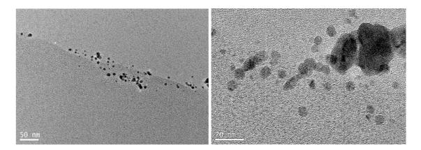
**Figure 2.** Transmission electron microscope images of a cross section of the palladium–crossbred wool nanocatalysts for S2 with different magnifications showing the Pd particles on the surface of the wool fiber. Similar TEM images were obtained for the other Pd–merino wool nanocatalysts.
