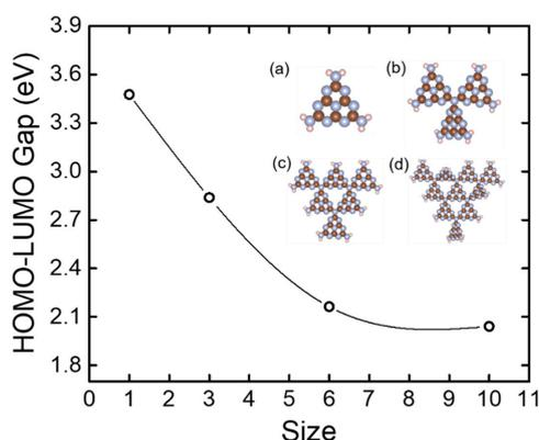
**Figure 1.** Calculated HOMO–LUMO gap vs  $g\text{-C}_3\text{N}_4$  structures with varying sizes. Insets show the optimized configurations of (a)  $g\text{-C}_3\text{N}_4\text{-1}$ ; (b)  $g\text{-C}_3\text{N}_4\text{-3}$ ; (c)  $g\text{-C}_3\text{N}_4\text{-6}$ ; and (d)  $g\text{-C}_3\text{N}_4\text{-10}$ . Brown, blue, and pink spheres represent C, N, and H, respectively.
