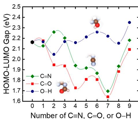
**Figure 2.** Calculated HOMO–LUMO gap vs a  $g-C_3N_4-6$  structure with varying numbers of  $C\equiv N$ ,  $C=O$ , and  $O-H$ . Configurations used for DFT calculations are shown in Figures 3–5. Insets show the functional groups in the calculated configurations. Brown, blue, pink, and red spheres represent C, N, H, and O, respectively.
