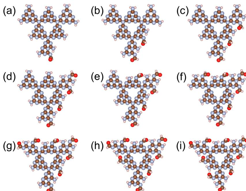
**Figure 4.** Structures of  $g\text{-C}_3\text{N}_4\text{-6}$  with varying numbers of  $\text{C}=\text{O}$  groups. Brown, blue, pink, and red spheres represent C, N, H, and O, respectively.
