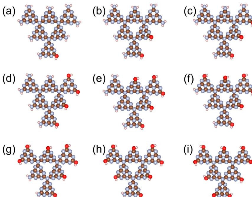
**Figure 5.** Structures of  $g\text{-C}_3\text{N}_4\text{-6}$  with varying numbers of  $\text{O}-\text{H}$  groups. Brown, blue, pink, and red spheres represent C, N, H, and O, respectively.
