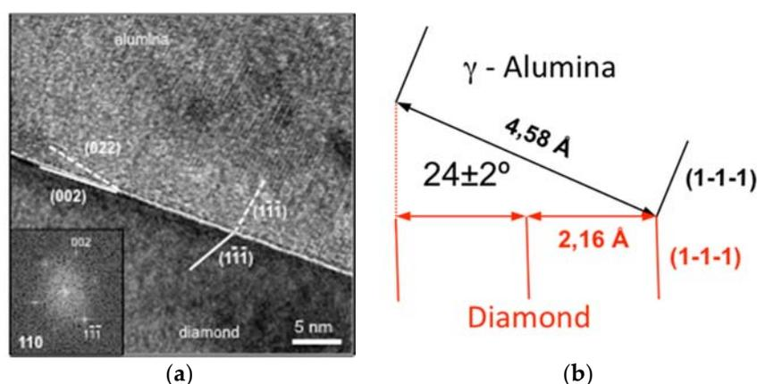
**Figure 4.** (a) HREM micrograph of sample C, where a fully crystalline alumina layer is observed. Lines and dashed lines were used to indicate where the  $(\bar{1}\bar{1}\bar{1})$  planes are in both diamond and alumina crystals. The insets correspond to the FFTs of both materials; (b) Schematic representation of the  $(\bar{1}\bar{1}\bar{1})$  planes' correspondence at the diamond/alumina interface in sample C.
