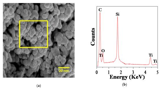
**Figure S4.** Field emission scanning electron microscopy with energy dispersive X-ray (FESEM-EDX) measurements (a) Micrograph of selected image; and (b) Energy dispersive X-ray (EDX) spectrum collected from (1)Ti-SiNS.
