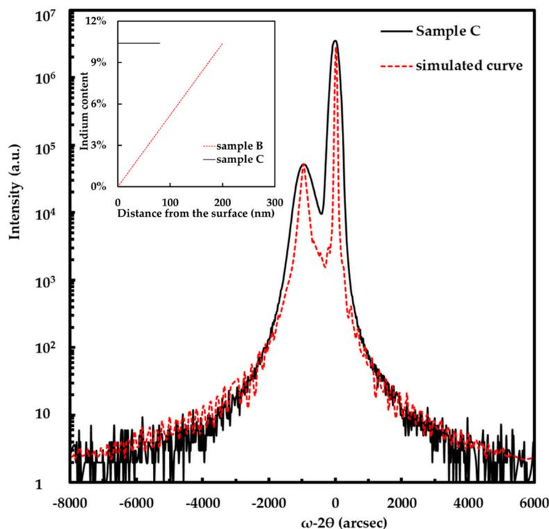
**Figure 2.** High-resolution X-ray diffraction  $\omega$ -2 $\theta$  scan of sample C. The dashed line in red is the simulated curve. The inset shows the indium content profiles of samples B and C.
