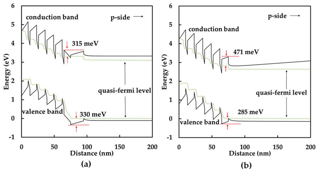
Figure 4. Calculated energy band diagrams at 300 mA of (a) sample A; and (b) sample B.
