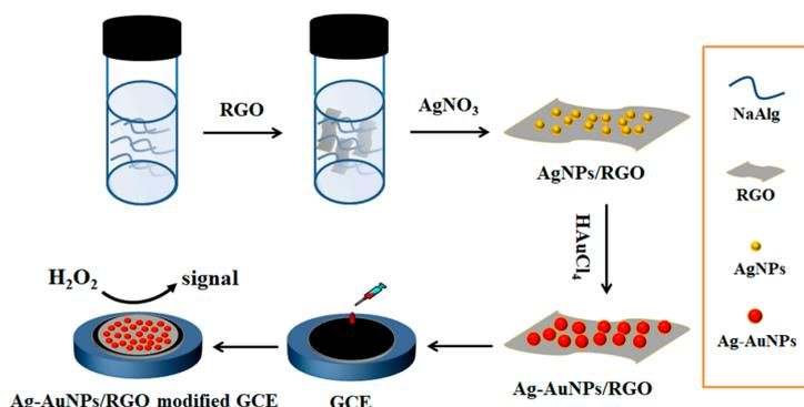
**Scheme 1.** Schematic illustration of synthesis of Ag-AuNPs/reduced graphene oxide (RGO) and its application in the electrochemical detection of H<sub>2</sub>O<sub>2</sub>.
