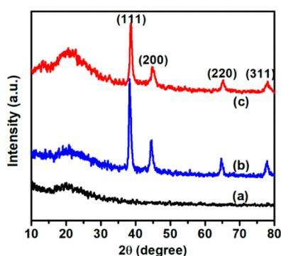
**Figure 3.** X-ray diffraction (XRD) patterns of RGO (a); AuNPs/RGO (b); and Ag-AuNPs/RGO (c).
