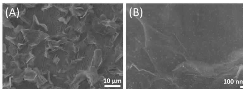
**Figure 1.** Scanning electron microscope (SEM) images of Ag-AuNPs/RGO magnified 1500 times (A); and 33,000 times (B).
