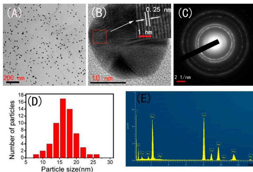
**Figure 2.** (A) Transmission electron microscopy (TEM) image; (B) HR-TEM image; (C) selected area electron diffraction (SAED) pattern; (D) the size distribution histogram; and (E) energy dispersive X-ray spectroscopy (EDS) spectrum of Ag-AuNPs/RGO.
