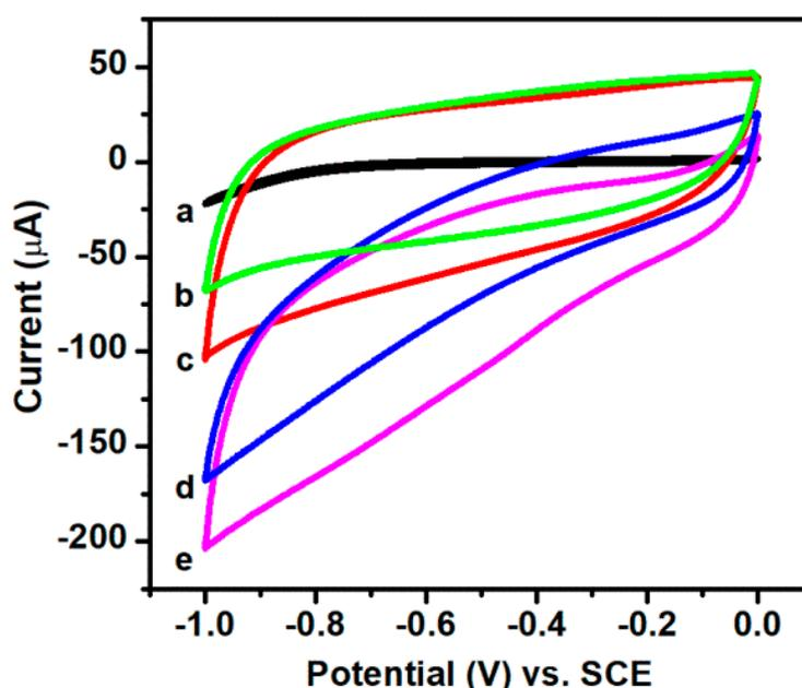
**Figure 5.** Cyclic voltammetry (CV) curves of bare GCE obtained in the presence of 3 mM  $\text{H}_2\text{O}_2$  (a); CV curves of AuNPs/RGO modified electrode obtained in the absence (b) and presence of 3 mM  $\text{H}_2\text{O}_2$  (d); and Ag-AuNPs/RGO modified electrode in the absence (c) and presence of 3 mM  $\text{H}_2\text{O}_2$  (e). Scan rate:  $50 \text{ mV} \cdot \text{s}^{-1}$ .
