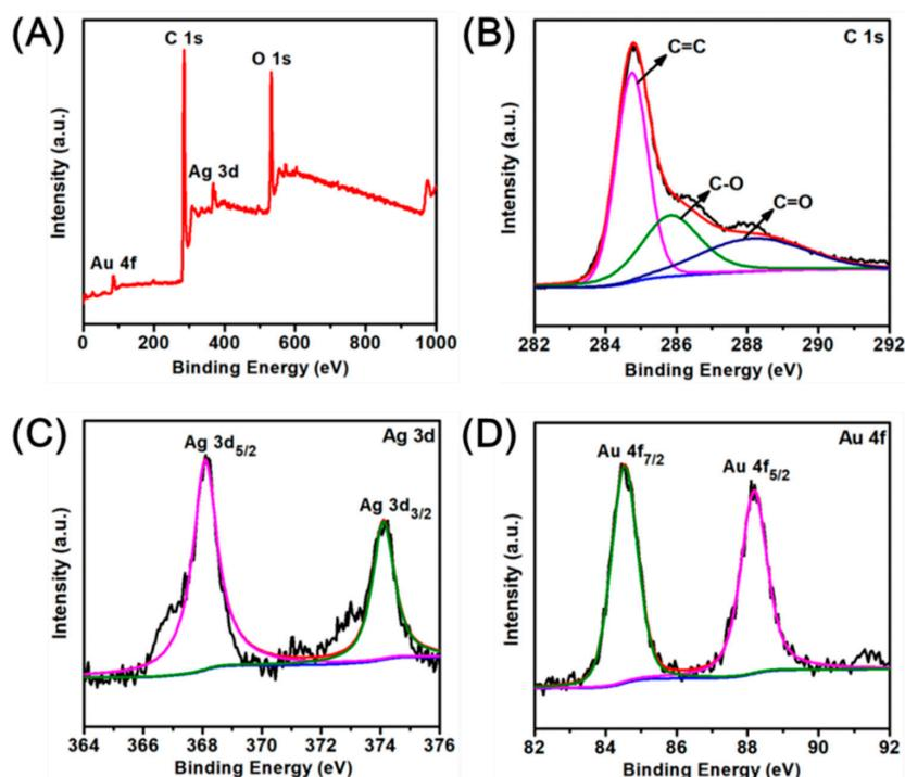
**Figure 4.** (A) X-ray photoelectron spectroscopy (XPS) full scan spectrum of Ag-AuNPs/RGO; (B–D) high resolution XPS spectrum for C 1s; Ag 3d; and Au 4f, respectively.
