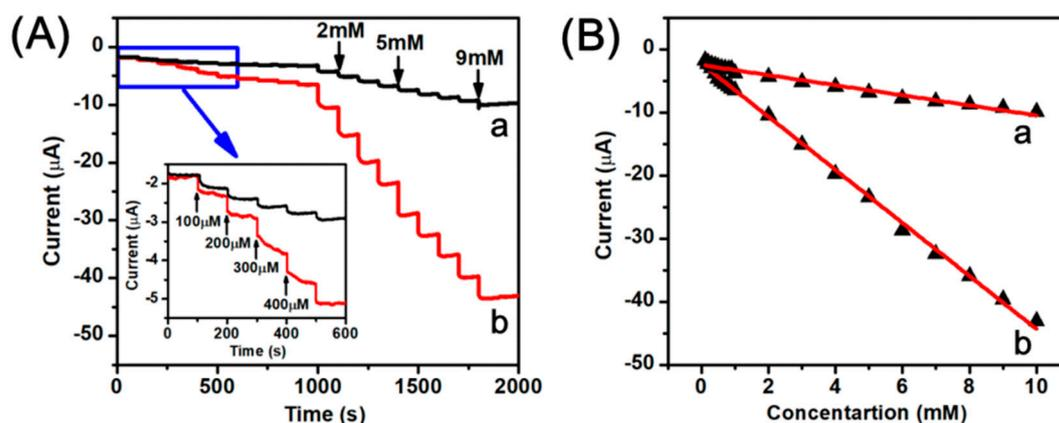
**Figure 7.** (A) Amperometric response of the AuNPs/RGO (a) and the Ag-AuNPs/RGO (b) sensors upon successive addition of H<sub>2</sub>O<sub>2</sub> into 0.1 M PBS, pH 7.2 under a stirring condition, applied potential  $-0.2$  V. The inset was the amplification of curve with the lower concentration region; (B) The linear relationship between different H<sub>2</sub>O<sub>2</sub> concentration and reduction current.
