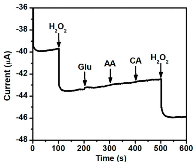
**Figure 8.** Amperometric response of the Ag-AuNPs/RGO modified GCE for the successive addition of  $\text{H}_2\text{O}_2$ , glucose, AA and CA (1 mM, respectively) in Ar-saturated 0.1 M PBS (pH 7.2) at  $-0.2$  V.
