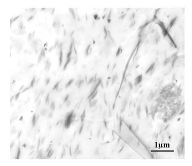
**Figure 2.** Transmission electron microscopy (TEM) image of the nanorubber highlighting the dispersed and intercalated structure of the layered silicates.
