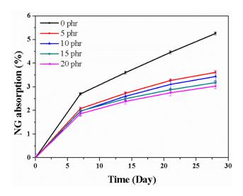
Figure 5. Nitroglycerin adsorption in EPDM/CR nanorubbers with various layered-silicate contents.
