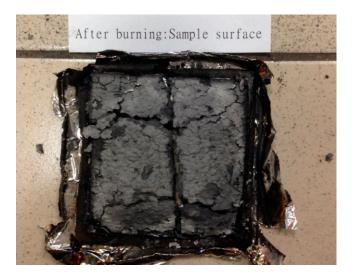
**Figure 7.** Photographic image showing char formation on an EPDM/CR nanorubber (10 phr layered silicates) after burning.
