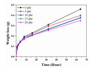
Figure 4. Triacetin-permeation in EPDM/CR nanorubbers with various layered-silicate contents.
