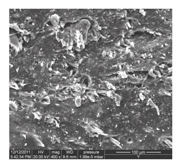
Figure 3. Scanning electron microscopy (SEM) image of a fractured surface of the EPDM/CR nanorubber.
