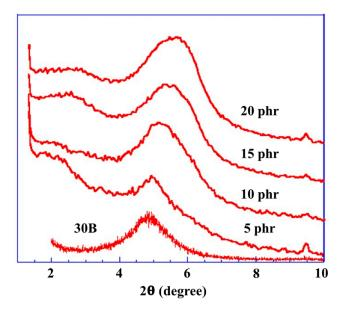
**Figure 1.** X-ray diffraction patterns of ethylenepropylenediene monomer/chloroprene rubber (EPDM/CR) nanorubbers with various layered-silicate contents.
