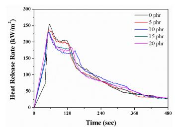
**Figure 6.** Typical heat release rate (HRR) curves for EPDM/CR nanorubbers with various layered-silicate contents.
