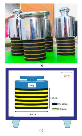
**Figure 8.** (a) Images of test specimens used in the nitroglycerine (NG)-migration and absorption experiments; (b) Illustration depicting the experimental set up for NG-migration and absorption experiments.
