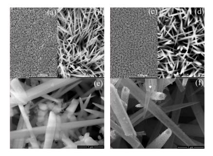
Figure 3. SEM images for  $(Ni,Co)_2(CO_3)(OH)_2$  nanorods (a,b,e) and  $NiCo_2S_4$  nanotubes (c,d,f) on Ti-PF.
