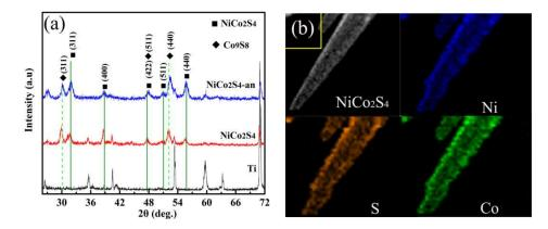
**Figure 5.** (a) XRD images for Ti-PF, NiCo<sub>2</sub>S<sub>4</sub>, and NiCo<sub>2</sub>S<sub>4</sub>-an on Ti-PF; (b) TEM image and the corresponding EELS elemental mapping images of a single NiCo<sub>2</sub>S<sub>4</sub> nanotube.
