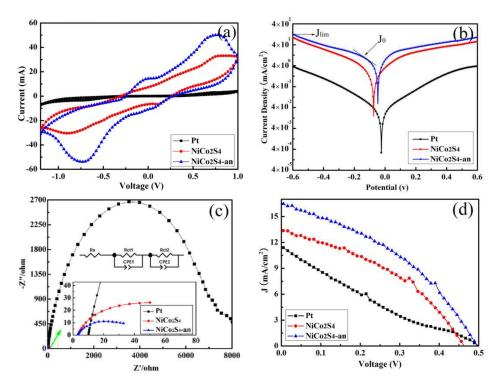
Figure 6. (a) Cyclic voltammetry (CV); (b) Tafel curves; and (c) EIS of the symmetric cells with Pt, NiCo<sub>2</sub>S<sub>4</sub>, and NiCo<sub>2</sub>S<sub>4</sub>-an CEs and (d) J–V characteristics for QDSSCs based on Pt, NiCo<sub>2</sub>S<sub>4</sub>, and NiCo<sub>2</sub>S<sub>4</sub>-an CEs, respectively.
