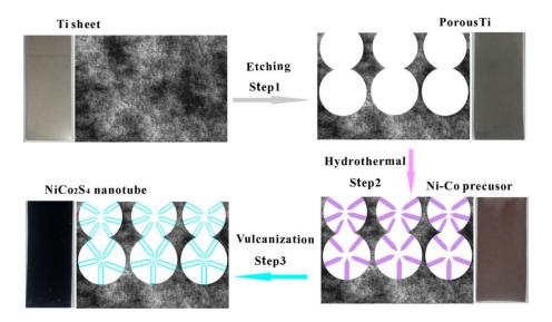
**Figure 1.** Schematic diagram to illustrate the preparation process of  $NiCo_2S_4$  nanotubes on Ti porous film (Ti-PF).
