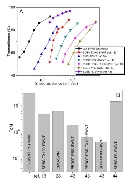
**Figure 9.** Comparison of electrical properties of rGO-SWNT film with those films contained other dispersing agents. (A) Transmittance versus sheet resistance profiles; (B) Comparison of figure of merit (FoM) CMC: sodium carboxymethyl cellulose; SDS: sodium dodecyl sulphate; FS: fluorosurfactant (FC-4430).
