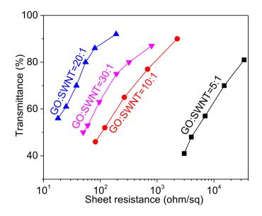
**Figure 7.** Sheet resistance versus optical transmittance for rGO-SWNT films fabricated from inks with different GO to SWNT mass ratios. The SWNT content in the ink is 0.2 mg/mL.
