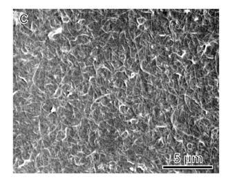
**Figure 5.** SEM micrographs of rGO-SWNT films prepared from inks with different GO to SWNT mass ratios: (**A**) 5:1, (**B**) 10:1 and (**C**) 20:1.
