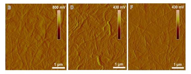
**Figure 8.** AFM height (**A**, **C** and **E**) and amplitude (**B**, **D** and **F**) micrographs of rGO-SWNT films prepared from inks with different GO to SWNT mass ratios: (**A**) 5:1, (**B**) 10:1 and (**C**) 20:1.
