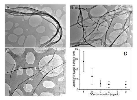
**Figure 2.** TEM micrographs of (**A**) SWNT bundles in water; (**B**) GO-SWNT dispersion with a GO:SWNT mass ratio of 10:1; (**C**) GO-SWNT dispersion with a GO:SWNT mass ratio of 20:1. The concentration of SWNT in each case is 0.2 mg/mL; (**D**) Effect of GO concentration on the diameter of SWNT bundles in the dispersion. The SWNT content in the ink is 0.2 mg/mL.
