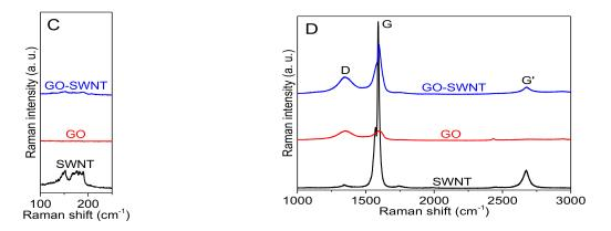
**Figure 1.** (**A**) UV-vis absorbance of diluted GO and GO-SWNT (weight ratio of 10:1) dispersions. Pure SWNT solution (weakly oxidized by nitric acid) is shown for comparison. The inset photo displays GO-SWNT (left) and GO (right) dispersions. (**B**) Absorbance of GO-SWNT dispersion for different time periods. (**C**,**D**) Raman profiles of GO-SWNT dispersion (weight ratio of 10:1), GO and SWNT.
