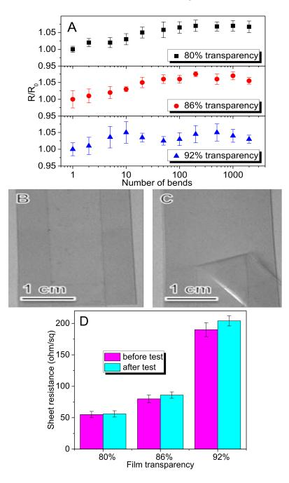
**Figure 10.** (**A**) Relative sheet resistance vs. benching cycles for rGO-SWNT films.  $R_0$  is the electrical resistance of samples before bending, and R is the electrical resistance that changes with bending cycles. Error bars reflect standard deviation for five measurements; (**B**,**C**) Mechanical stability of rGO-SWNT/PET film: before and after the Scotch tape test; (**D**) Sheet resistance vs. transparency before and after Scotch tape peeling test.
