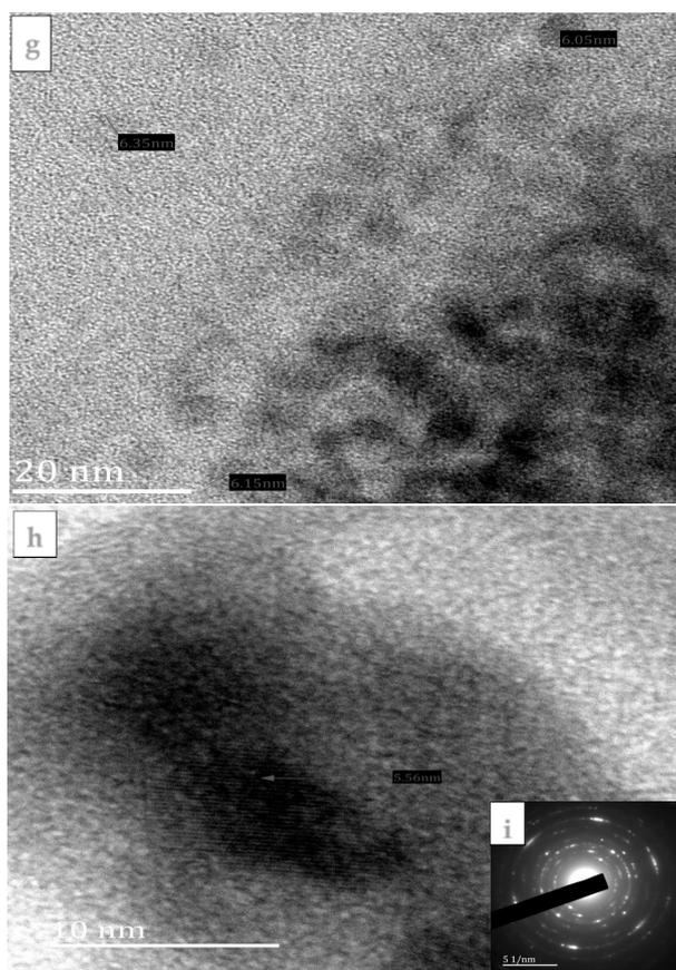
**Figure 2.** HRTEM image (a) lattice fringe (b) and SAED pattern (c) of FeS1 nanoparticles; HRTEM image (d) lattice fringe (e) and SAED pattern (f) of FeS2 nanoparticles; HRTEM image (g) lattice fringe (h) and SAED pattern (i) of FeS3 nanoparticles.
