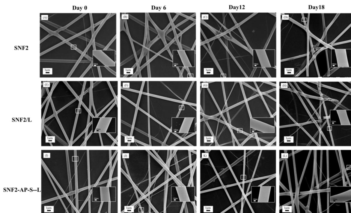
**Figure 5.** SEM images of SNF2 (A–D), SNF2/L (E–H), and SNF2-AP-S-L (I–L) after being immersed in 10 mM PBS with daily buffer exchange for different time periods at 37 °C. (A,E,I) at Day 0, (B,F,J) at Day 6, (C,G,K) at Day 12, (D,H,L) at Day 18. Scale bars represent 1  $\mu\text{m}$  in (A–L) and 100 nm for the insets.
