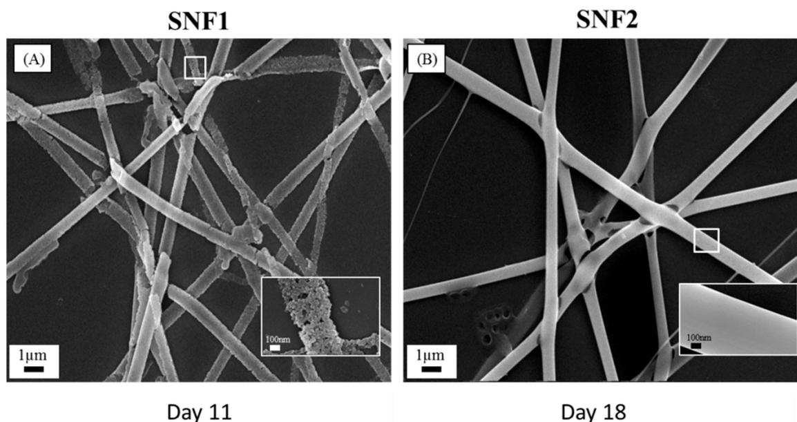
**Figure 2.** Scanning electron microscope (SEM) images of (A) SNF1 immersed in 10 mM PBS with daily buffer exchange at 37 °C after 11 days and (B) SNF2 immersed in 10 mM phosphate-buffered saline (PBS) with daily buffer exchange at 37 °C after 18 days. The insets are the magnification of the corresponding surfaces. The scale bars represent 1  $\mu\text{m}$  in (A,B) and 100 nm for the insets.
