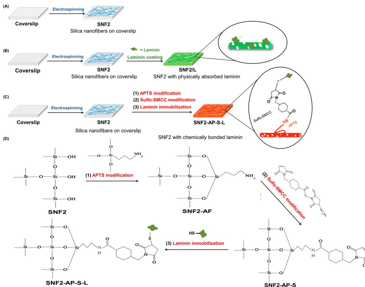
**Figure 1.** Schematic of the surface modifications of the three SNF2 substrates. (A) Silica nanofibers (SNF2) electrospun onto coverslip; (B) physically laminin-adsorbed SNF2 (SNF2/L) (C) chemically laminin-bonded SNF2 (SNF2-AP-S-L); (D) the chemical reactions for the preparation of SNF2-AP-S-L.
